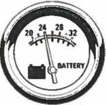
**Voltmeter:** Indicates electrical system voltage. With engine operating, normal reading should be 24-27.5 volts.
