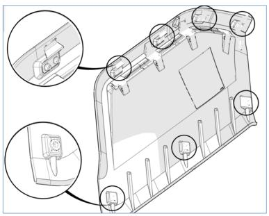
FIGURE 2: ATTACHMENT POINTS AT THE BACK OF THE PANEL
