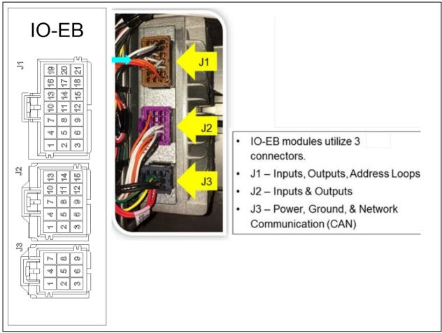
FIGURE 12: I/O-EB MODULES CONNECTOR PIN-OUT - BACK PROBING VIEW
