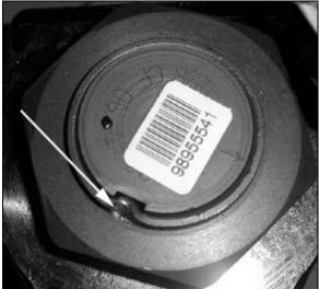
FIGURE 20: FIXING NUT PUNCH MARK
