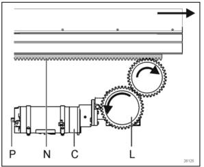
FIGURE 48 EXTENSION MOTOR GEARS (FORE SHOWN)
