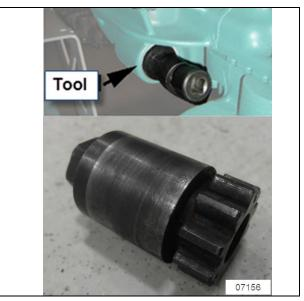
FIGURE 10: VOLVO ENGINE TURNING TOOL #88800014
