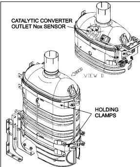
FIGURE 5: CATALYTIC CONVERTER
