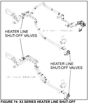
FIGURE 74: X3 SERIES HEATER LINE SHUT-OFF VALVES
