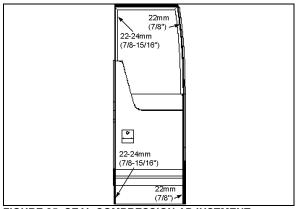
FIGURE 25: SEAL COMPRESSION ADJUSTMENT 18632
