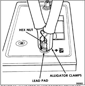
FIGURE 30: ALLIGATOR CLAMP POSITION STANDARD BATTERY
