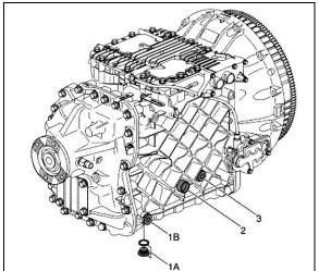
FIGURE 17: I-SHIFT TRANSMISSION OIL CHANGE
