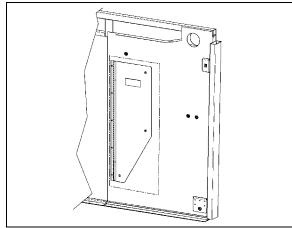
FIGURE 19: PASSENGER'S UNIT 2-PART AIR FILTER ACCESS PANEL
