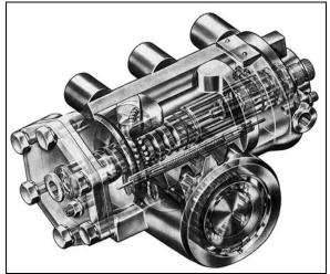
FIGURE 3: POWER STEERING GEAR
