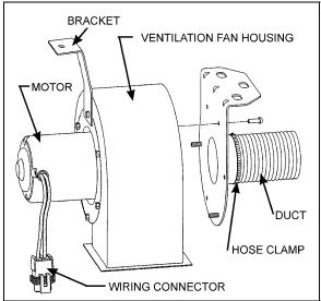
FIGURE 24: VENTILATION FAN INSTALLATION 23222
