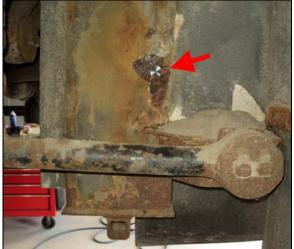
FIGURE 6: CLEANED SPOT ON STRUCTURAL MEMBER
