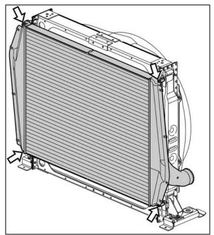
FIGURE 32: SEPARATING CHARGE AIR COOLER
