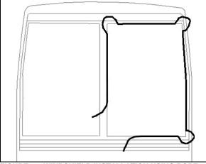
FIGURE 57: WINDSHIELD INSTALLATION USING ROPE
