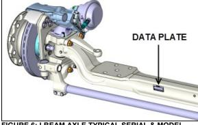
FIGURE 6: I-BEAM AXLE TYPICAL SERIAL & MODEL NUMBERS 00008
