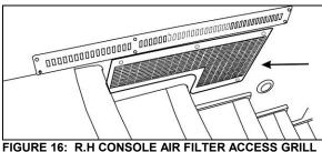
FIGURE 16: R.H CONSOLE AIR FILTER ACCESS GRILL (COACHES) 18505
