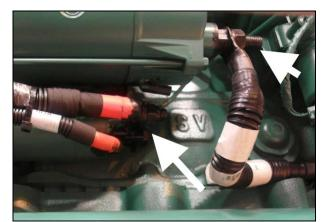
Figure 26: Starter power cable and ground cable lugs protected with Color Guard rubber coating.
