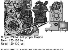
Single 5VX940 belt to 3rd alternator proper tension Automatic with pneumatic bellows FIGURE 24: BELT LAYOUT WITH 3RD ALTERNATOR
