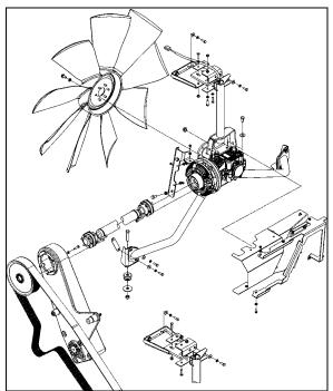
FIGURE 36: COOLING FAN DRIVE MECHANISM 05149
