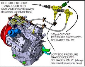
FIGURE 30: PRESSURE TRANSDUCERS
