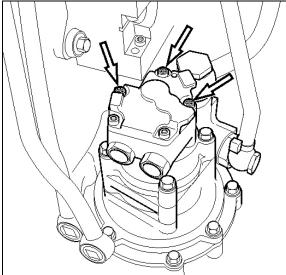
FIGURE 6: FUEL PUMP REMOVAL
