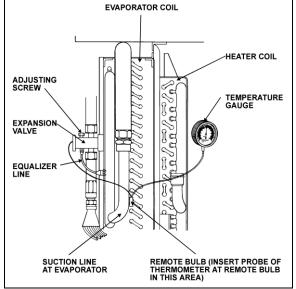
FIGURE 51: SUPERHEAT ADJUST. INSTALLATION 22046
