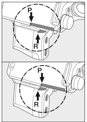
FIGURE 25: PAD WEAR CHECK FRONT AND TAG AXLE
