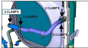
FIGURE 8: COOLANT LINE AT THE RADIATOR OUTLET
