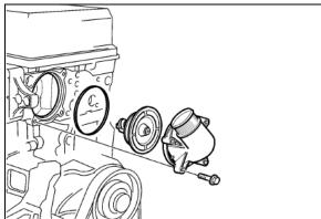
FIGURE 5: VOLVO D13 THERMOSTAT HOUSING
