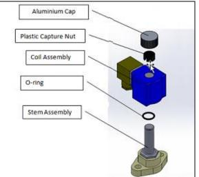
FIGURE 32: UNLOADER COIL ASSEMBLY
