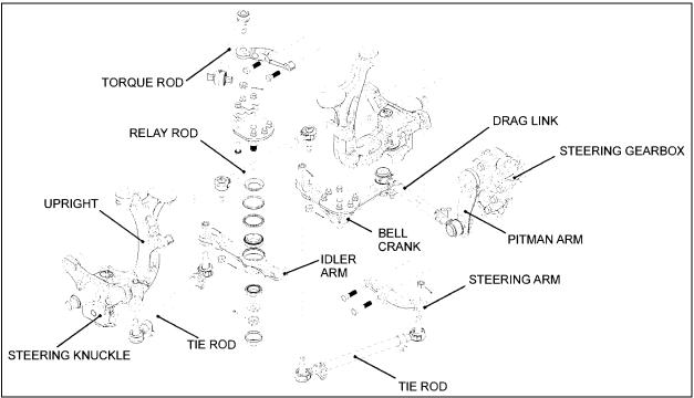
FIGURE 10: IFS STEERING LINKAGE OVERVIEW
