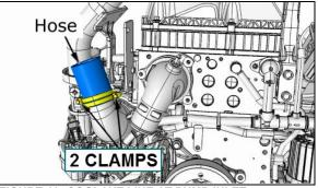
FIGURE 10: COOLANT LINE AT PUMP INLET
