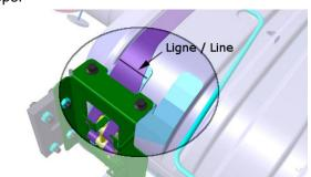
Mark, with a vertical line the central position of the lower and upper clamps with regard to the emboss located at the bottom and at the top of the catalytic converter.
