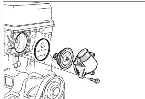
FIGURE 13: VOLVO D13 THERMOSTAT HOUSING
