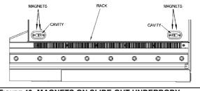
FIGURE 40: MAGNETS ON SLIDE-OUT UNDERBODY
