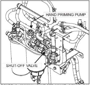
FIGURE 2: MANUAL SHUT-OFF VALVE (VOLVO D13 ENGINE) 03088\_2
