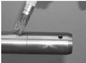
FIGURE 10: APPLY GLEITMO 805 GREASE
