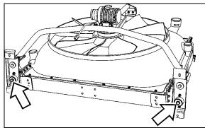
FIGURE 33: REMOVING FASTENERS
