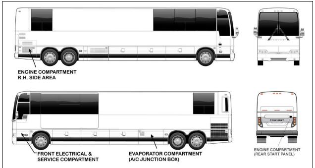
FIGURE 7: ELECTRICAL COMPARTMENTS (X3-45 VIP COMMERCIAL BUS SHELL)
