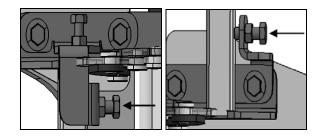
To adjust door depth, loosen the screws fixing the hinge to frame assembly and slide the hinge horizontally to move the door in or out. Depth should be calculated at 29mm +/-2mm measured from bus frame out or 5mm +1mm if measurement is taken from small square tube on frame.
