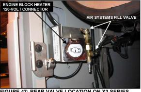
FIGURE 47: REAR VALVE LOCATION ON X3 SERIES
