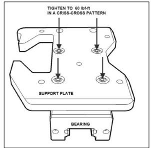
FIGURE 24: BEARING MOUNTING SCREWS
