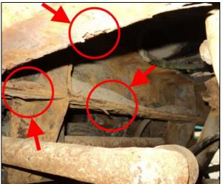
FIGURE 3: METAL FLAKING AND ACCUMULATED SAND
