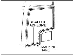
FIGURE 37: ADHESIVE-MOUNTED WINDOW 18081
