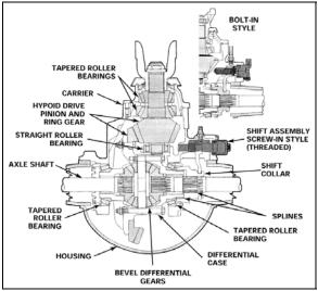
FIGURE 3: DRIVER-CONTROLLED DIFFERENTIAL LOCK
