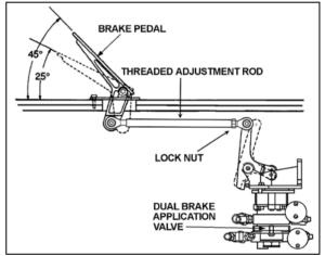
FIGURE 14: BRAKE PEDAL ADJUSTMENT
