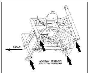
FIGURE 80: JACKING POINTS ON FRONT UNDERFRAME – IFS
