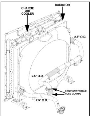
FIGURE 2: COOLANT FLOW TO RADIATOR (VOLVO D13)
