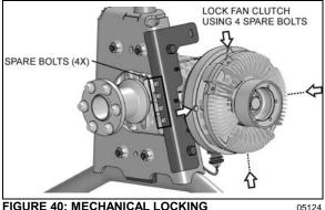
FIGURE 40: MECHANICAL LOCKING
