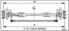
FIGURE 41: TOE-IN MEASUREMENT
