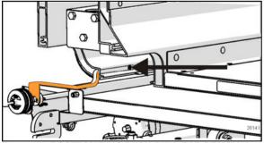
FIGURE 57: POSITION RING PUSH-PULL TAB REMOVAL.
