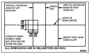
FIGURE 50: AIM INSPECTION LIMITS FOR UPPER-BEAM HEADLIGHTS
