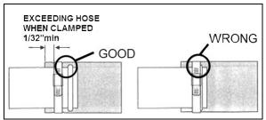
FIGURE 3: PROPER HOSE CLAMP INSTALLATION
