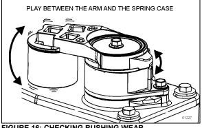
FIGURE 16: CHECKING BUSHING WEAR
