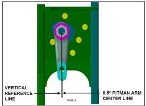
FIGURE 35: IFS PITMAN ARM ALIGNMENT
