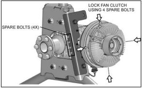
FIGURE 24: MECHANICAL LOCKING
