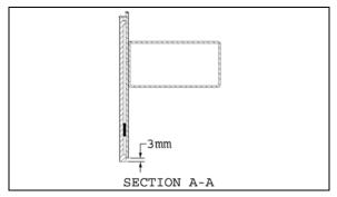
• Line-up body panel with window. There must be a gap of 4±2mm between window and body panel.
