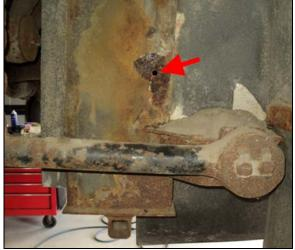
FIGURE 7: HOLE DRILLED IN STRUCTURAL MEMBER
