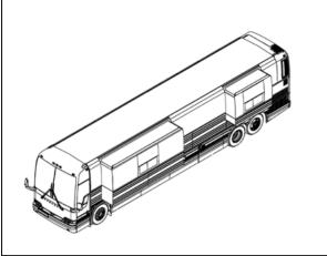
FIGURE 1: X3-45 VIP TYPICAL CONFIGURATION X3-45 VIP can be fitted with up to two slide-outs. (Figure 1)
