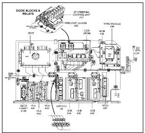
FIGURE 20: FRONT ELECTRICAL AND SERVICE COMPARTMENT
