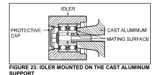
4. Bolt the new idler on the cast aluminum support.
