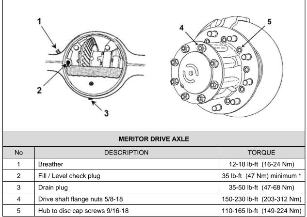
\* Minimum value, tighten until only one full plug thread is visible.
