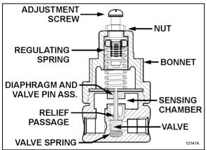
FIGURE 8: AIR PRESSURE REGULATING VALVE
