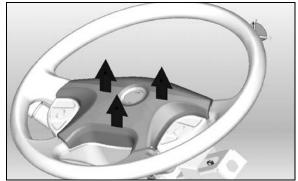
FIGURE 11: REMOVING THE HORN PAD
