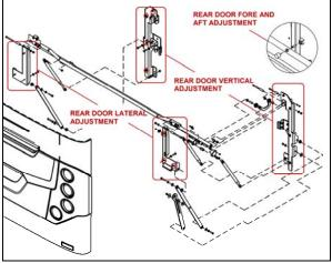
FIGURE 70: ENGINE COMPARTMENT DOOR 18633\_1
