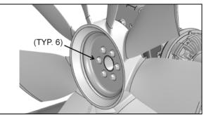
FIGURE 41: RADIATOR FAN MOUNTING BOLTS 05125
