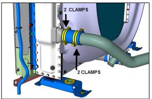
FIGURE 6: COOLANT LINE TO THE RADIATOR
