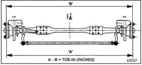
FIGURE 5: TOE-IN MEASUREMENT
