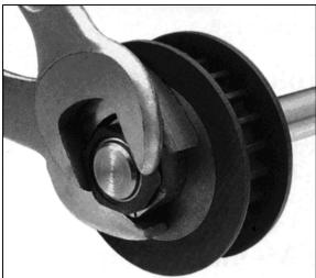
FIGURE 16: KEYLESS BUSHING TIGHTENING
