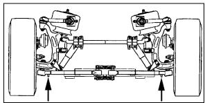
FIGURE 83: JACKING POINTS ON IND. SUSPENSION
