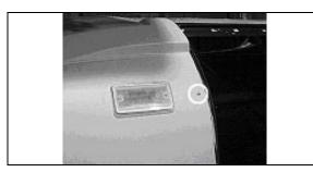
Apply a double-face self adhesive tape 1/8 by ¼ inch inside the molding onto the whole length.
