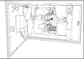
FIGURE 14: EVAPORATOR COIL CLEANING WITH LOW-PRESSURE AIR JET 22373
