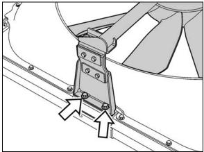
FIGURE 34: REMOVING UPPER FAN DRIVE SUPPORT BRACKET
