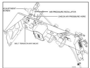
FIGURE 9: AIR PRESSURE REGULATOR (H-SERIES)
