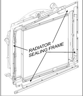
FIGURE 11: RADIATOR SEALING FRAME
