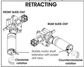
FIGURE 41: SLIDE-OUT MOTOR ROTATION
