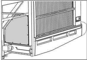
FIGURE 22: ACCESS PANEL BEHIND TAG AXLE WHEEL
