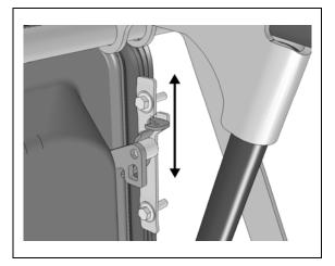
6. Open baggage compartment door and adjust using the cylinder mounting block.
