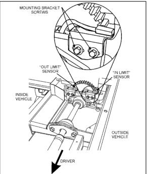
FIGURE 39: SLIDE-OUT SENSORS
