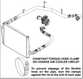
FIGURE 12: CHARGE AIR COOLER HOSE CLAMPS
