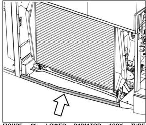
FIGURE 28: LOWER RADIATOR ASSY TUBE PROTECTOR
