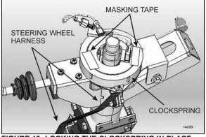
FIGURE 13: LOCKING THE CLOCKSPRING IN PLACE
