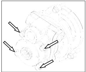
FIGURE 8: POWER STEERING PUMP REMOVAL
