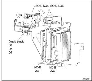
FIGURE 23 : PNEUMATIC ACCESSORY PANEL
