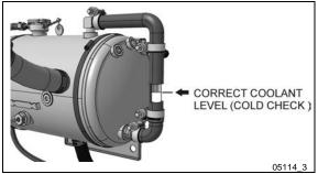
FIGURE 14: SURGE TANK IN ENGINE COMPARTMENT
