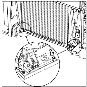
FIGURE 29: RADIATOR ASSEMBLY LOWER MOUNTING FASTENERS
