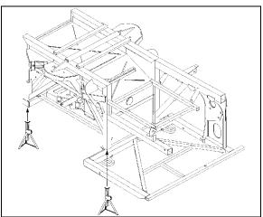
FIGURE 89: FRONT END JACKING POINTS 18592
