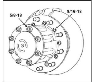
FIGURE 9: FASTENER SIZE IDENTIFICATION
