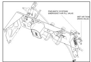
FIGURE 46: REAR VALVE LOCATION ON H3 SERIES 12162
