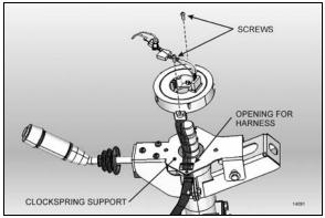
FIGURE 14: CLOCKSPRING INSTALLATION
