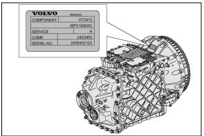
FIGURE 3: I-SHIFT TRANSMISSION
