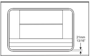
FIGURE 25: SLIDE-OUT LEVEL ADJUSTMENT
