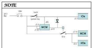
JB6 is a wake-up pin. JA15 output remains active for 5 minutes after JB6 is inactive.
