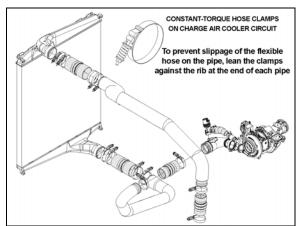
FIGURE 4: CHARGE AIR COOLER HOSE CLAMPS
