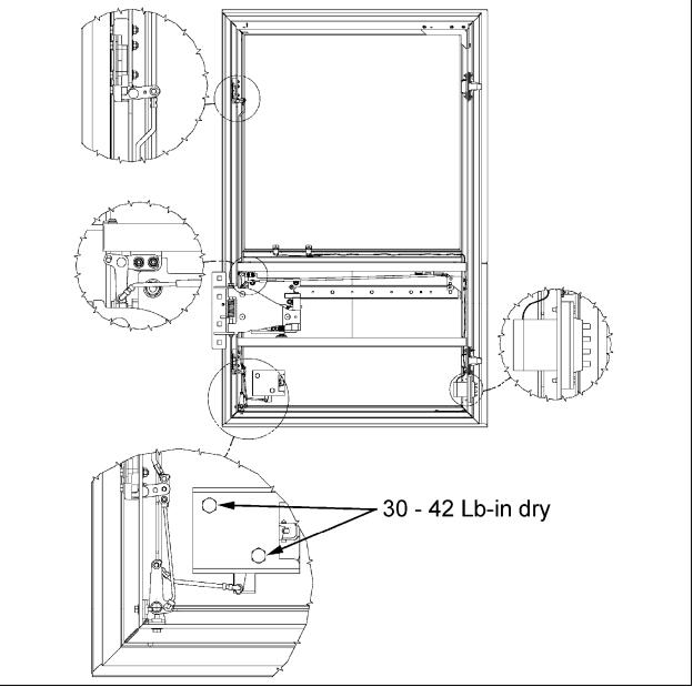
FIGURE 55: WCL SLIDING DOOR OPENING MECHANISM
