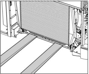
FIGURE 17: POSITIONING FORKLIFT
