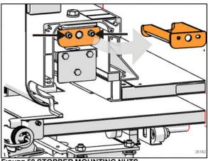
FIGURE 58 STOPPER MOUNTING NUTS
