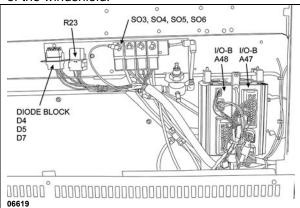
FIGURE 15: ENTRANCE DOOR & WIPER CONTROL PANEL
