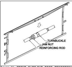
FIGURE 11: FRONT SLIDE-OUT ROOF REINFORCING
