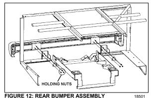
3. To install bumper, reverse the procedure.
