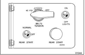
FIGURE 21: ENGINE REAR START PANEL
