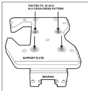
FIGURE 24: BEARING MOUNTING SCREWS
