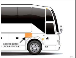
FIGURE 54: ACCESS TO LEVELING SCREWS, FORE
