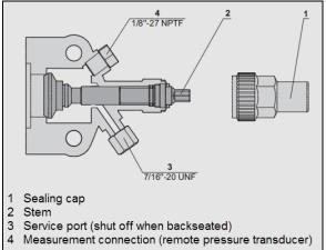
FIGURE 78: COMPRESSOR SHUT-OFF VALVE IN FRONT SEATED POSITION
