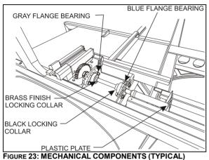
There are two different types of flange bearing on the slide-out mechanism (Figure 23). Their purpose is to maintain the shaft in position while permitting rotation. The gray flange bearings are fixed to the linear bearing support plate and are not adjustable. The blue flange bearings are fixed to a support with oblong holes allowing vertical adjustment to follow the linear bearing support plate position as it is being adjusted.
