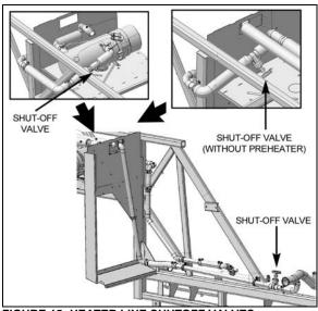
FIGURE 15: HEATER LINE SHUTOFF VALVES 05144
