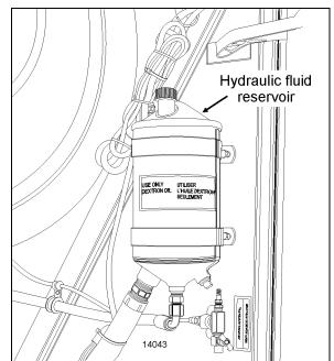
FIGURE 25: HYDRAULIC FLUID RESERVOIR LOCATION
