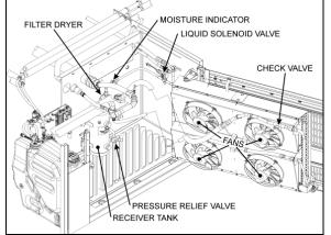
FIGURE 41: X3 SERIES CONDENSER COMPARTMENT22299
