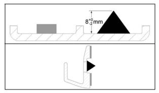
Position and fix vertical molding. Lean vertical molding against lateral molding. Make sure vertical molding lines up with structural tubing.
