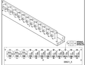
FIGURE 2: TYPICAL REAR ELECTRICAL JUNCTION PANEL – X3 SERIES
