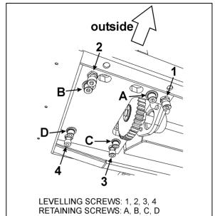
FIGURE 26: SLIDE-OUT LEVELING
