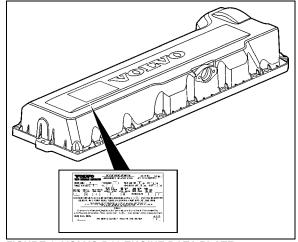
FIGURE 1: VOLVO D13 ENGINE DATA PLATE
