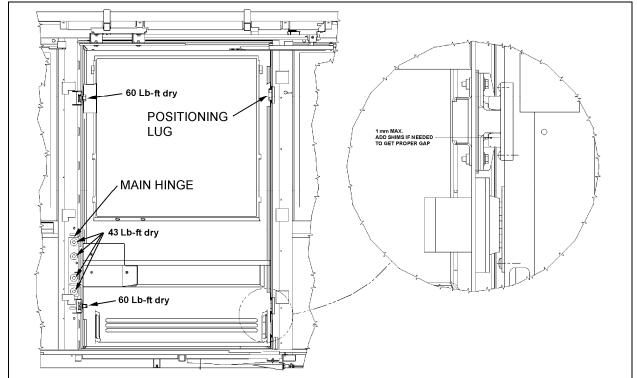
FIGURE 52: WCL SLIDING DOOR INSTALLATION
