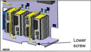
FIGURE 36: IO-B MODULE REMOVAL
