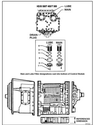
FIGURE 7: DRAIN PLUG AND FILTERS
