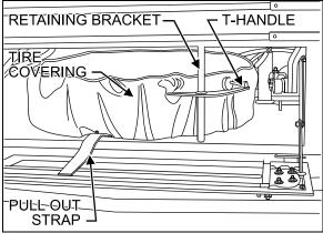
FIGURE 29: X3 SERIES SPARE WHEEL AND TIRE 18415
