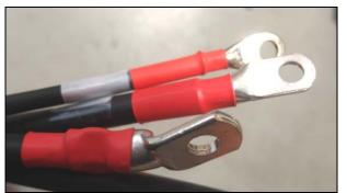
Figure 13: Cable lugs must be closed type, crimped or welded.
