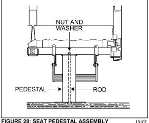
FIGURE 28: SEAT PEDESTAL ASSEMBLY
