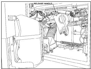
FIGURE 11: FRONT BUMPER RELEASE HANDLE 18613
