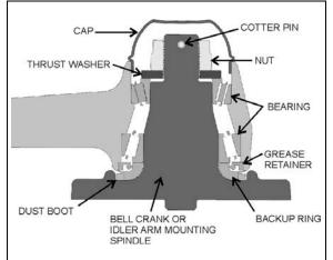
FIGURE 14: BELL CRANK OR IDLER ARM HUB
