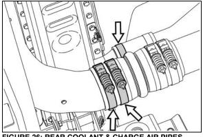
FIGURE 26: REAR COOLANT & CHARGE AIR PIPES
