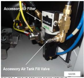
FIGURE 3: FRONT SERVICE COMPARTMENT
