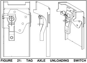
FIGURE 21: TAG AXLE UNLOADING SWITCH ADJUSTMENT 14061
