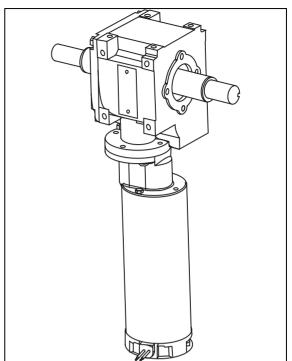
FIGURE 19: ELECTRIC MOTOR AND SPEED REDUCTION GEARBOX
