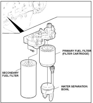
FIGURE 5: FUEL FILTERS WITH VOLVO D13 ENGINE
