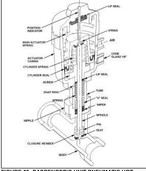
FIGURE 53: PASSENGER'S UNIT PNEUMATIC HOT WATER VALVE 22241
