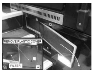
FIGURE 17: REMOVING DRIVER'S SECTION AIR FILTERS
