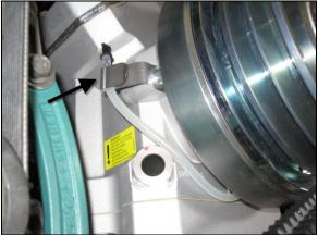
FIGURE 31: SHAFT SEAL OIL COLLECTING TUBE
