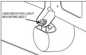
FIGURE 65: FOG LIGHT MOUNTING BOLT
