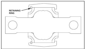
FIGURE 30: UPPER A-ARM BALL PIN BUSHING
