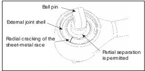
FIGURE 7: BALL PIN BUSHING
