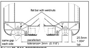
FIGURE 28: RAIL POSITIONING
