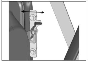
Check handle adjustment. Handle must 5. remain tight against its plastic housing.
