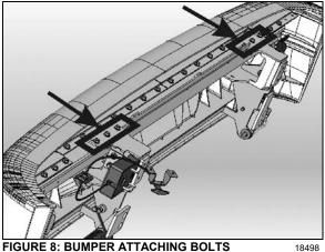
FIGURE 8: BUMPER ATTACHING BOLTS 18498 To reinstall the front bumper, reverse the procedure.
