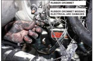
Figure 22: Fire in engine compartment caused by rubbing of power cable against metal edge of Bosch T1 alternator rear cover. Lower rubber grommet was missing when fire occured. Evidence of electrical arc can be seen.
