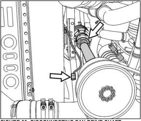
FIGURE 30: DISCONNECTING FAN DRIVE SHAFT
