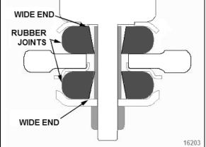
FIGURE 42: LOWER SHOCK MOUNTING BUSHINGS
