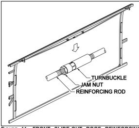
FIGURE 11: FRONT SLIDE-OUT ROOF REINFORCING ROD
