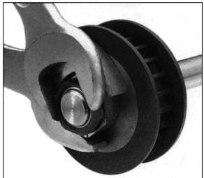
FIGURE 16: KEYLESS BUSHING TIGHTENING
