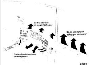
FIGURE 61: DRIVER'S UNIT AIR CIRCULATION
