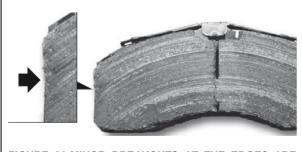
FIGURE 26:MINOR BREAKOUTS AT THE EDGES ARE PERMITTED (SEE ARROW)
