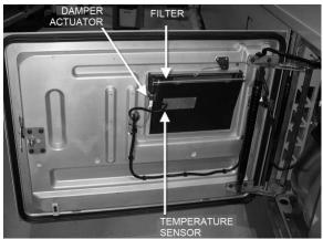
FIGURE 62: X3 SERIES PASSENGERS' AREA FRESH AIR DAMPER 22302\_A
