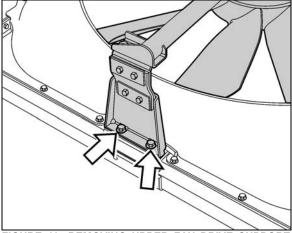
FIGURE 19: REMOVING UPPER FAN DRIVE SUPPORT BRACKET
