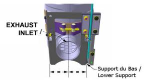
• While tightening the bolts, keep in mind to respect the alignment of the parts and keep the lower support as centered as possible with the catalytic converter exhaust inlet.
