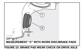
If measurement "C" is less than 0.039" (1 mm), this condition requires a check of the brake pad thickness and the brake disc with the wheel removed. If any minimal tolerance limits have been reached, the pads and/or disc must be changed.
