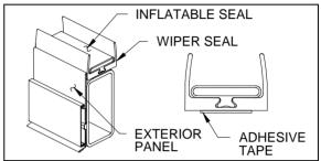
FIGURE 33: SEAL ASSEMBLY
