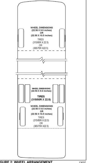
FIGURE 2: WHEEL ARRANGEMENT
