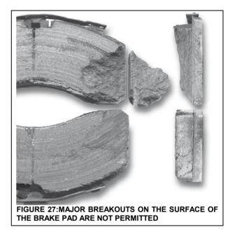
If the thickness of the friction material at its thinnest point is less than 0.079 inch or 2 mm (measurement C), the pads must be replaced.
