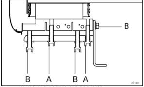
FIGURE 53: TILT AND LEVELING SCREWS
