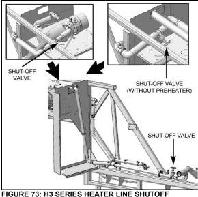
FIGURE 73: H3 SERIES HEATER LINE SHUTOFF VALVES 05144
