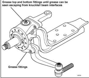
FIGURE 2: FRONT AXLE GREASING POINTS
