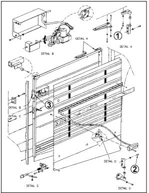
FIGURE 73: ENGINE COMPARTMENT R.H. SIDE DOOR18635
