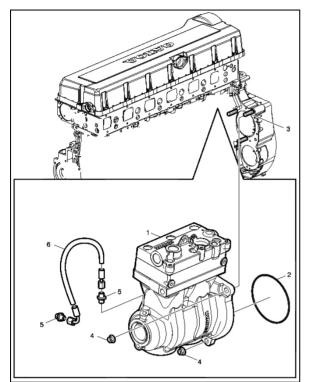
FIGURE 10: AIR COMPRESSOR LOCATION 03061
