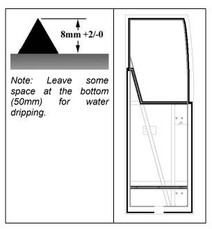
• Install and center fiber glass body panel onto door frame leaving an excess of 3mm all around the frame.
