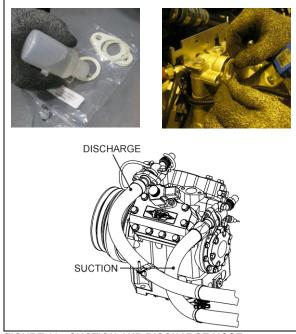
FIGURE 29: SUCTION AND DISCHARGE HOSE
