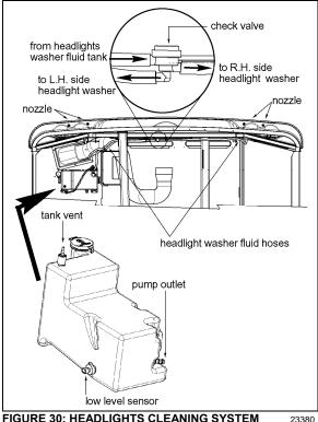
FIGURE 30: HEADLIGHTS CLEANING SYSTEM
