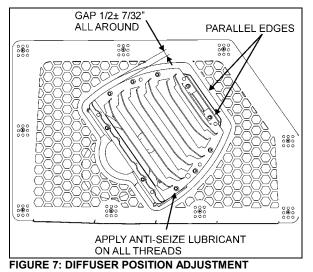
2. For proper angular position, make sure that the two edges shown on figure 7 are parallel with each other.
