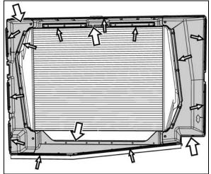
FIGURE 24: RADIATOR SEALING FRAME
