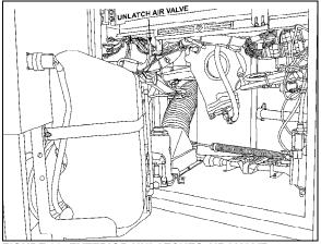
FIGURE 22: EXTERIOR UNLATCHES AIR VALVE 12209
