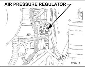
FIGURE 14: AIR PRESSURE REGULATOR (TYPICAL)
