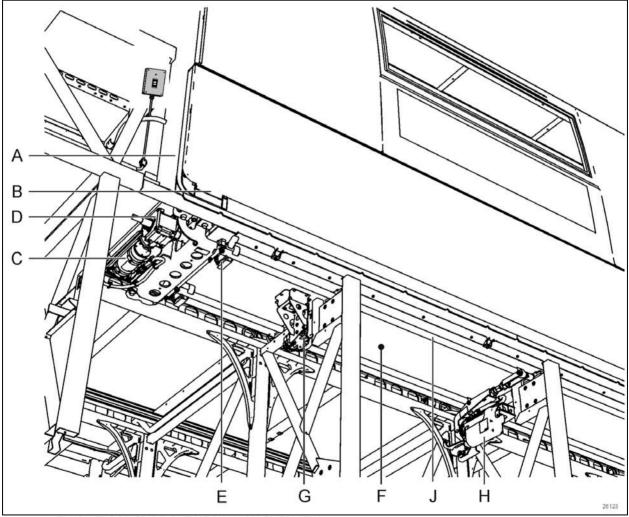
FIGURE 45: FLUSH FLOOR SLIDE-OUT MECHANISM OVERVIEW
