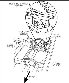
FIGURE 39: SLIDE-OUT SENSORS
