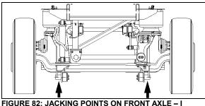
FIGURE 82: JACKING POINTS ON FRONT AXLE – I BEAM AXLE 10000
