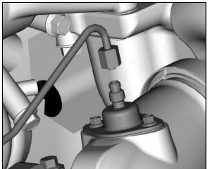
FIGURE 13: AFTERTREATMENT HYDROCARBON DOSER
