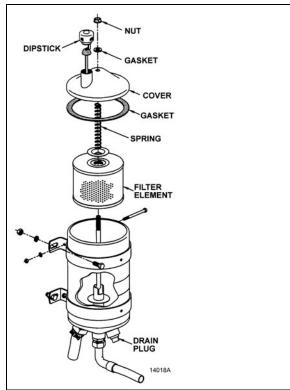
FIGURE 26: POWER STEERING FLUID RESERVOIR
