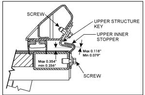
FIGURE 6: UPPER INNER STOPPERS ADJUSTMENT
