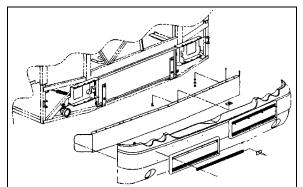
FIGURE 13: FRONT BUMPER REMOVAL
