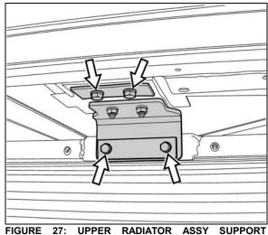
FIGURE 27: UPPER RADIATOR ASSY SUPPORT BRACKET
