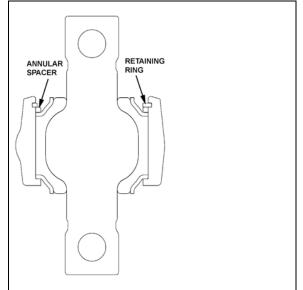
FIGURE 29: LOWER A-ARM BALL PIN BUSHING 16047
