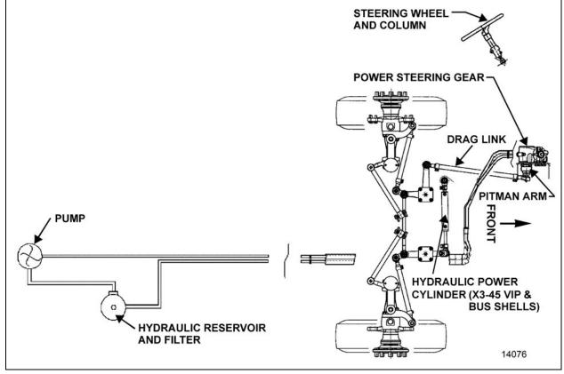
FIGURE 2: IFS STEERING SYSTEM SETUP
