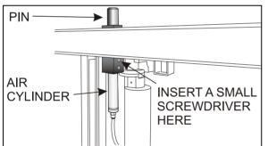
FIGURE 10: SECURITY PIN AIR CYLINDER REMOVAL
