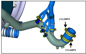
FIGURE 7: COOLANT LINE CONNECTED TO PUMP OUTLET
