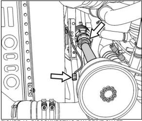
FIGURE 16: DISCONNECTING FAN DRIVE SHAFT
