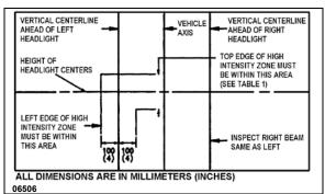
FIGURE 51: AIM INSPECTION LIMITS FOR LOWER-BEAM HEADLIGHTS
