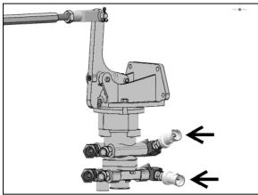
FIGURE 15: STOPLIGHTS PRESSURE SWITCH 12139
