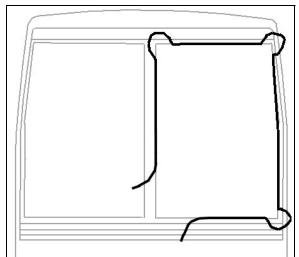
FIGURE 48: WINDSHIELD INSTALLATION USING ROPE
