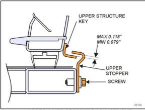
FIGURE 52: UPPER INNER STOPPERS ADJUSTMENT
