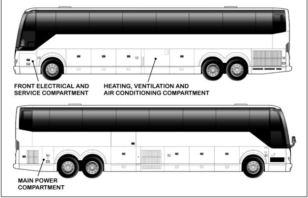
FIGURE 17: ELECTRICAL COMPARTMENTS
