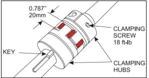
FIGURE 22: JAW COUPLING
