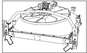
FIGURE 18: REMOVING FASTENERS
