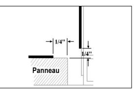
In the case of front finishing joint, apply some masking tape on each side of joint.
