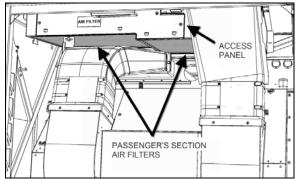
FIGURE 21: PASSENGERS' SECTION AIR FILTER 22375
