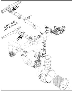
FIGURE 13: CHARGE AIR COOLER HOSE CLAMPS
