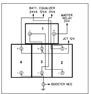
FIGURE 24 : H3 SERIES BATTERY CONNECTIONS (STANDARD ACID-LEAD GROUP 31)
