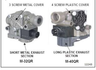
Mixing valve type on the left and right sides of the vehicle may result in slight pull to one side when braking.
