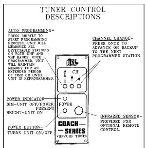
FIGURE 14: TUNER CONTROLS DESCRIPTION
