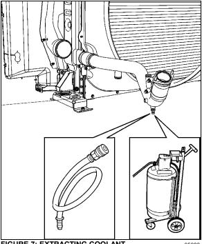
FIGURE 7: EXTRACTING COOLANT
