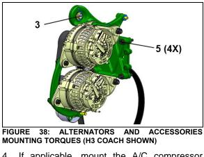
4. If applicable, mount the A/C compressor idler pulley onto alternator belt tensioner support (item 3). Use some Loctite 243 blue (680038) onto the threads.
