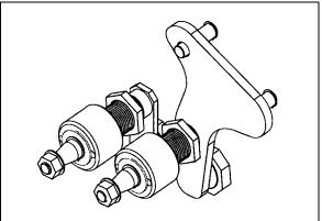
FIGURE 39: DRIVING MECHANISM (MOTOR SIDE) 23285
