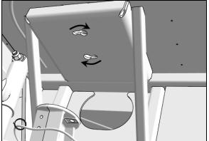
FIGURE 3: AIR SPRING UPPER MOUNTING PLATE
