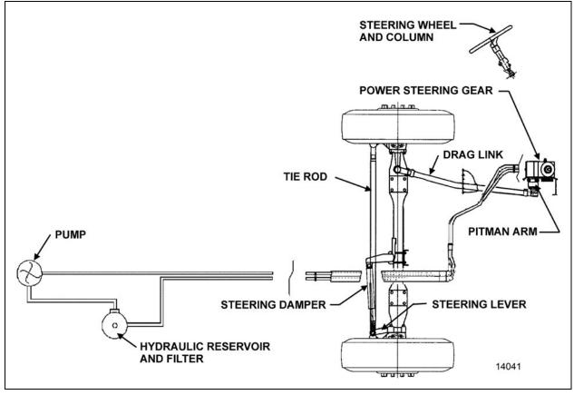
FIGURE 1: I-BEAM AXLE STEERING SYSTEM SETUP
