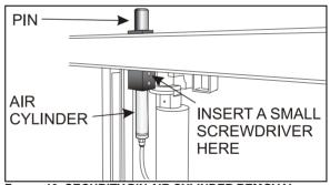
FIGURE 10: SECURITY PIN AIR CYLINDER REMOVAL
