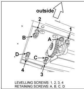
FIGURE 26: SLIDE-OUT LEVELING
