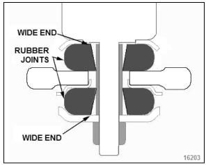
FIGURE 35: LOWER SHOCK MOUNTING BUSHINGS
