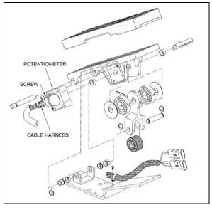
FIGURE 13: ELECTRONIC FOOT PEDAL ASSEMBLY 3035
