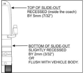
FIGURE 27: TILT ADJUSTMENT
