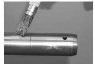
FIGURE 19: APPLY GLEITMO 805 GREASE
