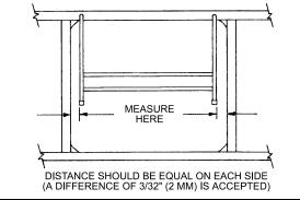
FIGURE 59: PANTOGRAPH DOOR ADJUSTMENT 18063
