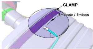
Using the lines made earlier, line up the lower and upper clamps with regard to the emboss of the converter and afterward, line up the lines made earlier on the clamps with regard to the clamp supports on the catalytic converter.
