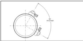
FIGURE 4: DOUBLED CLAMP POSITIONING
