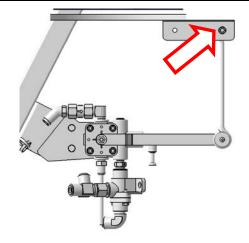
5. Loosen the lower mounting bolt shown.
