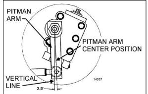
FIGURE 18: I-BEAM FRONT AXLE PITMAN ARM ADJUSTMENT
