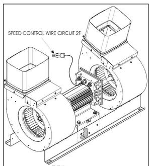
FIGURE 37: EVAPORATOR MOTOR ASSEMBLY
