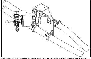
FIGURE 67: DRIVER'S UNIT HOT WATER PNEUMATIC VALVE ASSEMBLY
