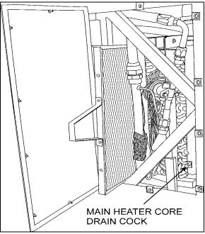
FIGURE 76: EVAPORATOR COMPARTMENT
