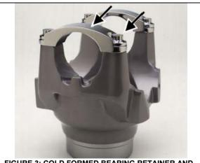
FIGURE 3: COLD FORMED BEARING RETAINER AND BOLTS AS USED ON PREVOST VEHICLES
