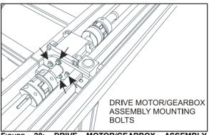
FIGURE 20: DRIVE MOTOR/GEARBOX ASSEMBLY MOUNTING BOLTS
