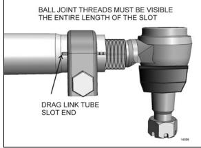
FIGURE 33: ADEQUATE CLAMPING CONDITION
