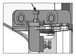
4. Using the 2 side adjusting screws (top and bottom), adjust door to get a 6mm to 8mm lateral gap (gap must be equal on both side).
