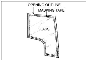
FIGURE 36: ADHESIVE-MOUNTED WINDOW
