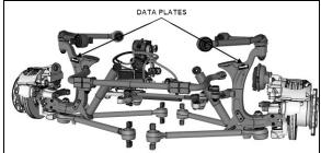
FIGURE 5: IFS TYPICAL SERIAL & MODEL NUMBERS
