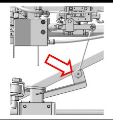
5. Loosen the lower mounting bolt shown.
