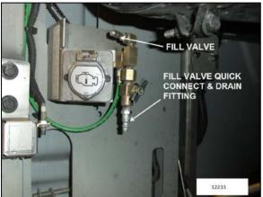
FIGURE 6: REAR VALVE LOCATION (typical)
