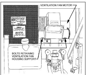
FIGURE 24: VENTILATION FAN INSTALLATION
