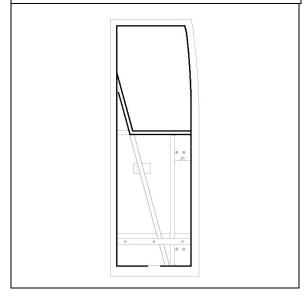
• Apply Sika 255 onto door frame structure.
