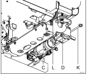
FIGURE 47: EXTENSION MOTOR (FORE SHOWN)
