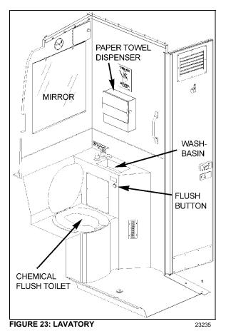
The lavatory has its own ventilation system that operates only when ignition switch is in the "ON" position.
