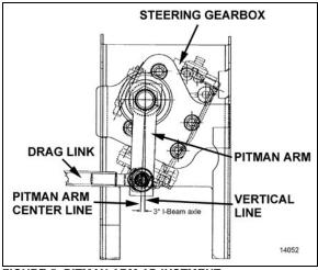
FIGURE 5: PITMAN ARM ADJUSTMENT
