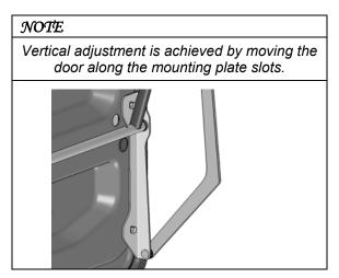
3. Center door in the opening using the retaining rings.
