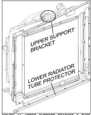
FIGURE 14: UPPER SUPPORT BRACKET & TUBE PROTECTOR
