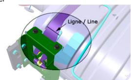
Before tightening the parts, make sure that the catalytic converter lower support is well centered with the exhaust inlet of the catalytic converter.
