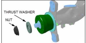
FIGURE 12: INSTALL THRUST WASHER AND HUB NUT
