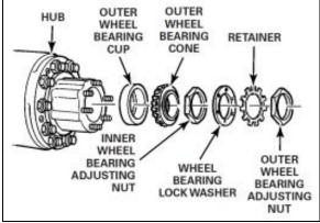
FIGURE 25: DRIVE AXLE WHEEL HUB
