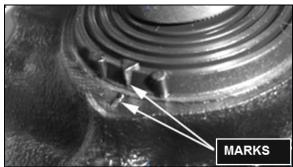
FIGURE 11: STEERING GEARBOX INPUT SHAFT MARKS
