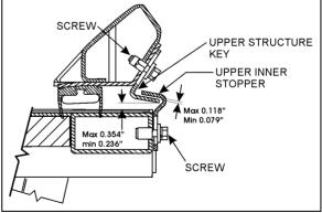
FIGURE 6: UPPER INNER STOPPERS ADJUSTMENT
