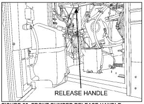
FIGURE 55: FRONT BUMPER RELEASE HANDLE 18613
