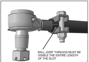
FIGURE 21: ADEQUATE CLAMPING CONDITION
