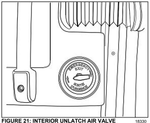
FIGURE 21: INTERIOR UNLATCH AIR VALVE
