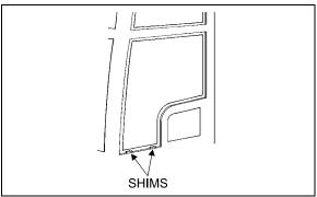
FIGURE 35: ADHESIVE-MOUNTED WINDOW
