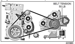
FIGURE 28: BELT LAYOUT WITH SMALL A/C COMPRESSOR
