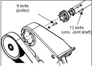
FIGURE 22: PULLEY AND SHAFT
