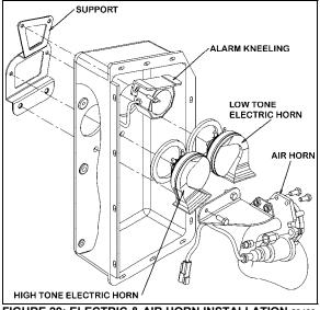
FIGURE 29: ELECTRIC & AIR HORN INSTALLATION 23420
