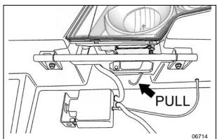
FIGURE 60: ROCKING THE HEADLIGHT ASSEMBLY
