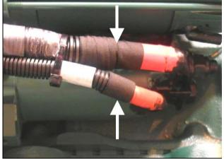
Figure 11: Two layers of fabric tape applied every 3 to 6 inches to prevent the cable from coming out of the corrugated protective sheath.
