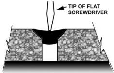
13. If welding was not performed properly, there will a loss of adhesion on one side. If this is the case, repair the joint.
