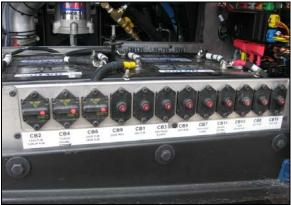
FIGURE 10: REAR ELECTRICAL JUNCTION PANEL
