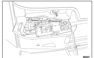
FIGURE 46: OPENING HEADLIGHT ASSEMBLY
