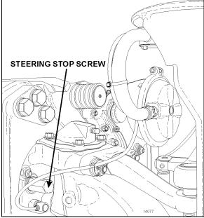
FIGURE 17: STEERING STOP SCREW ON I-BEAM AXLE
