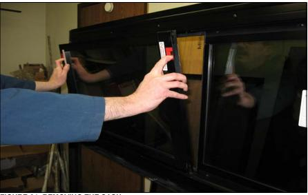
FIGURE 64: REMOVING THE SASH
