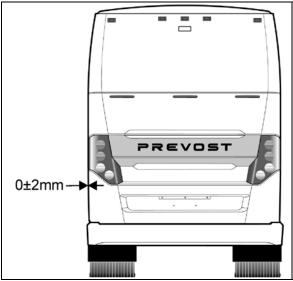
FIGURE 66: DOOR DEPTH ADJUSTMENT
