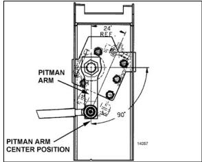
FIGURE 19: IFS PITMAN ARM ADJUSTMENT
