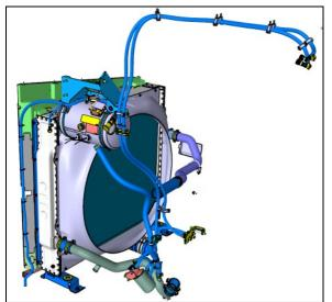
FIGURE 5: COOLANT FLOW TO RADIATOR (VOLVO D13)
