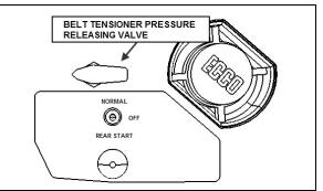
FIGURE 27: BELT TENSIONER CONTROL VALVE – X3 SERIES
