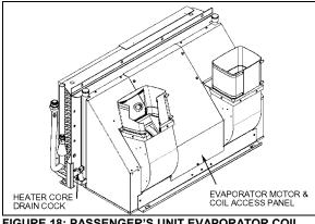
FIGURE 18: PASSENGER'S UNIT EVAPORATOR COIL
