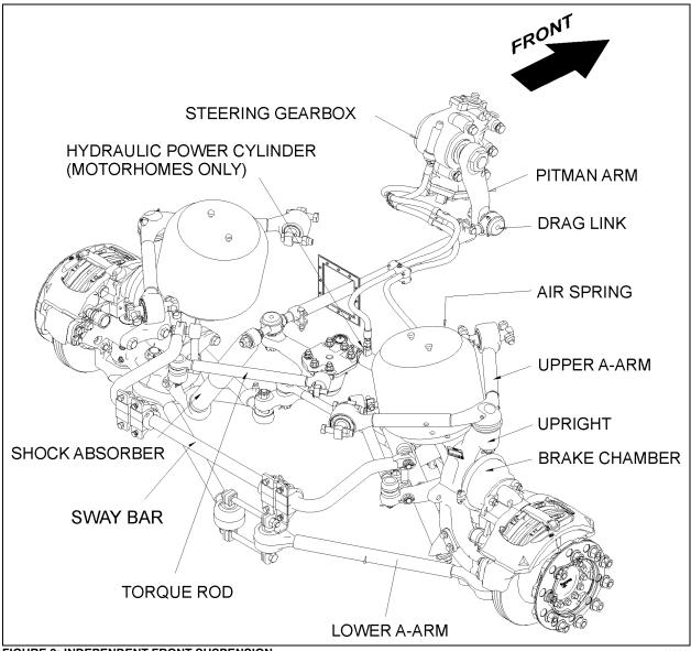
FIGURE 9: INDEPENDENT FRONT SUSPENSION
