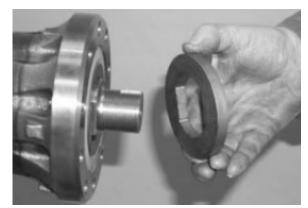
FIGURE 21: INSTALL THRUST WASHER
