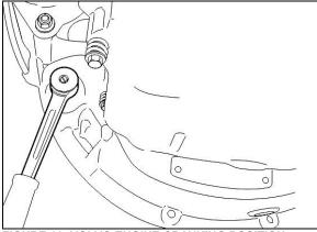
FIGURE 16: VOLVO ENGINE CRANKING POSITION
