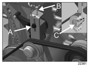
FIGURE 25: TENSIONER ON CENTRAL A/C
