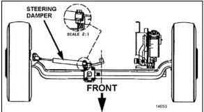
FIGURE 27: STEERING STABILIZER (DAMPER)
