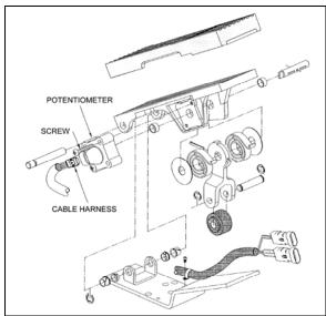
FIGURE 16: ELECTRONIC FOOT PEDAL ASSEMBLY 03035
