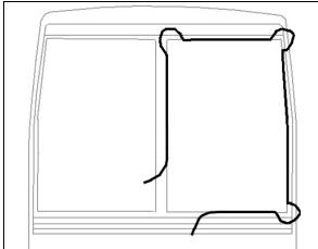
FIGURE 15: WINDSHIELD INSTALLATION USING ROPE
