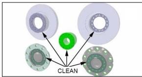
FIGURE 22: CLEANING HUB BEARING, ROTOR AND HUB FLANGE CLAMPING SURFACES
