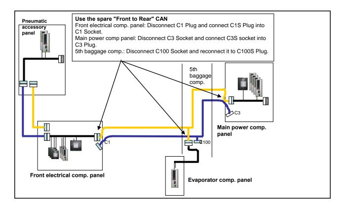
All modules including Wake-up modules and MCM have to be powered OFF prior to probe the CAN lines with an ohmmeter.
