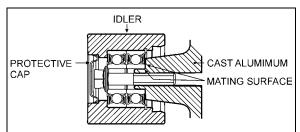
FIGURE 39: IDLER MOUNTED ON THE CAST ALUMINUM SUPPORT
