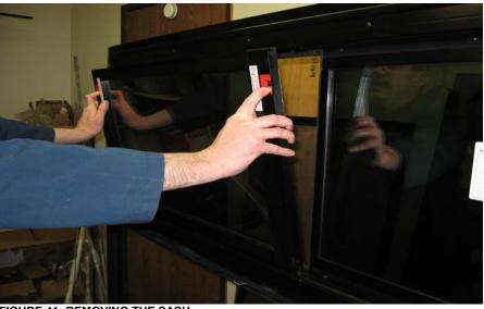
FIGURE 41: REMOVING THE SASH
