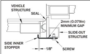
FIGURE 5: SIDE INNER STOPPER ADJUSTMENT
