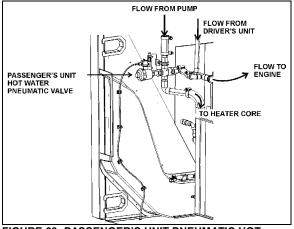
FIGURE 68: PASSENGER'S UNIT PNEUMATIC HOT WATER VALVE ASSEMBLY 22240
