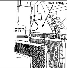
FIGURE 69: DRIVER'S HVAC/DEFROST UNIT
