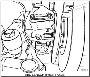
FIGURE 33: ABS SENSOR LOCATION
