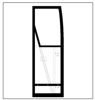
• Using a scratch pad "Scotch Brite", scratch the perimeter of the body panel where the adhesive will be applied.
