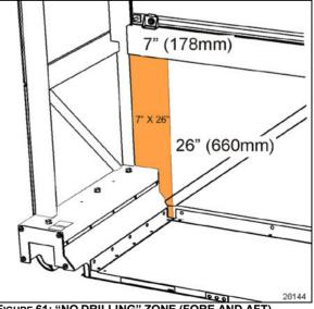
FIGURE 61: "NO DRILLING" ZONE (FORE AND AFT)
