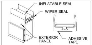
FIGURE 33: SEAL ASSEMBLY
