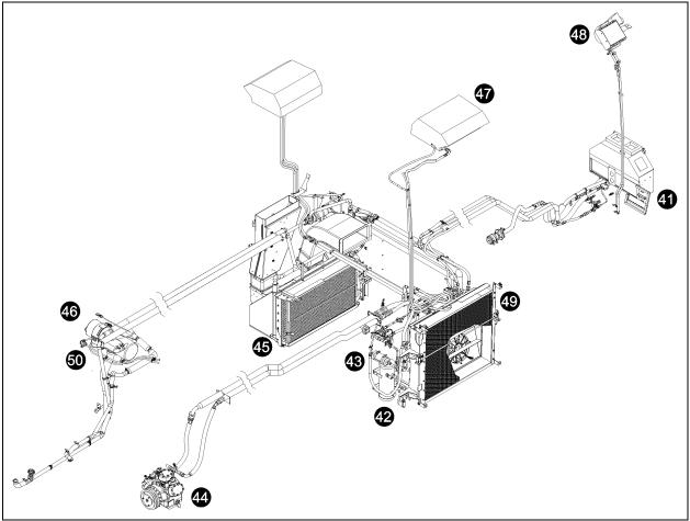
FIGURE 2: LUBRICATION AND SERVICING POINTS - HVAC UNIT
