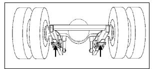
FIGURE 6: JACKING POINTS ON DRIVE AXLE H3B762
