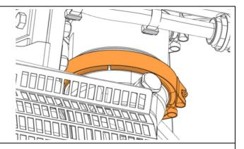
5. Grind off welding spatter of the DPF output.
