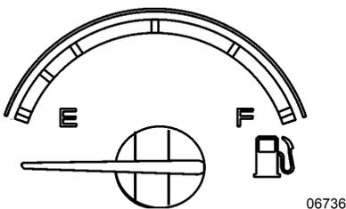
Indicates the amount of fuel remaining in the fuel tank. At the beginning of the red area, there is approximately 48 gallons (182 liters) left in the tank.
