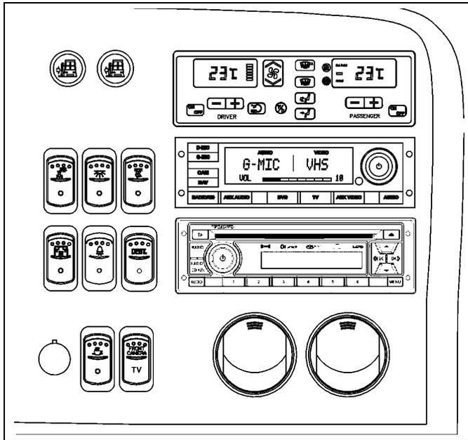
The HVAC control module as well as the cluster dimmer switch, interior lighting control switches, entrance door operating buttons as well as miscellaneous control switches and air vents are located on the R.H. dashboard panel.
