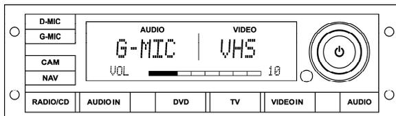
The VSS-05 Video and Sound Selector enables the driver to select audio, audio/video and video source with settings of volume level, bass, treble, etc. for the passenger's area only. The DVD player, TV tuner, P.A. system and auxiliary audio or video sources are controlled with this unit.
