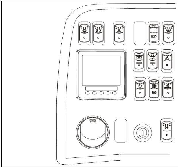
The L.H. dashboard panel includes controls for the operation of the coach; it also includes the ignition switch and an adjustable air vent.
