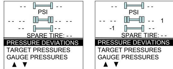
As illustrated, the pressure readings will appear replacing the dash lines as the TPMS display starts to receive pressure data from the TPMS receiver. It can take 1 minute to get all pressure readings updated since the sensors transmit at a one minute interval.
