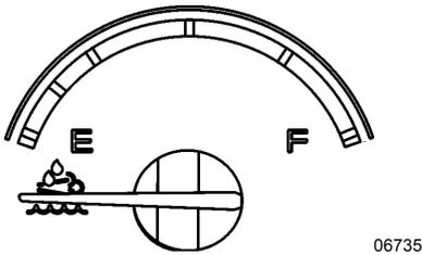
Indicates the amount of DEF (diesel exhaust fluid) remaining in the DEF tank. The DEF tank is considered as being full when it contains 16 gallons (60 liters) of DEF. DEF consumption will be approximately 2% of the diesel fuel consumed.
