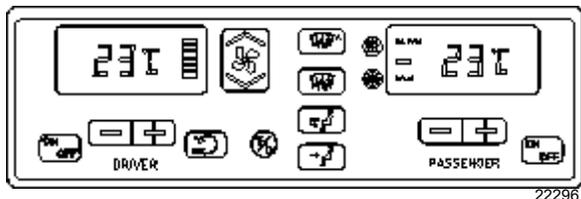
The vehicle is slightly pressurized by the central HVAC system to prevent dust and moisture from entering. Air flow and controls divide the vehicle into two areas: driver's area with defroster and passengers' area.
