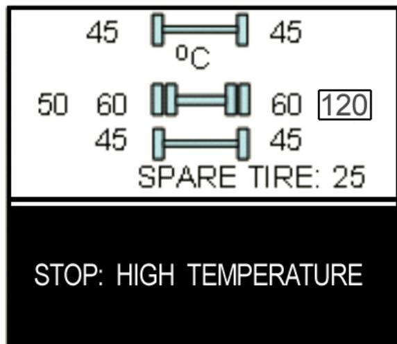
To get the driver's attention to the alarms, the bottom section of the screen where the alarm message appears will blink to reverse contrast
