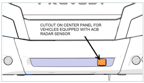
Figure 1: VEHICLE EQUIPPED WITH ACB RADAR SENSOR
