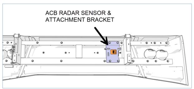
Figure 2: VEHICLE EQUIPPED WITH ACB RADAR SENSOR
