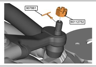
12. Adjust the drag link to the correct length 70mm (A) and fit it to the Pitman arm, checking that the steering gear is in the centre position. If not, adjust the drag link.
