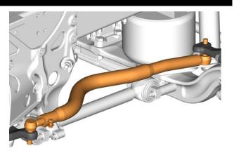
3. Remove castle nut and split pin the drag link from the steering arm and discard.
