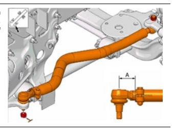
6. Torque screw and nut of the clamp to 170Nm.
