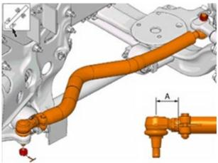
13. Torque screw and nut of the clamp to 170Nm.
