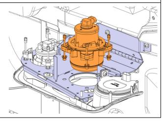
930040 8. Remove headlamp adjusters (3x) from new lamps 930040 (2x) and discard 9. Install new headlamp adjuster kit 930373 930040 (2x) on new lamps 930040(2x). 930373 10. Lock adjusters on lamps 11. Install new lamps modified with new 930040 adjuster on the support (both sides).
