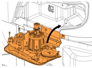
14. Secure lamp assembly with fixing screws **(both sides).**
