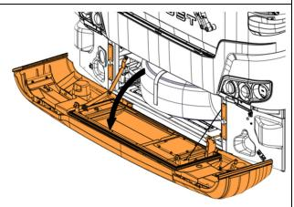
4. Unscrew fixing screws (both sides).
