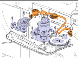
7. Remove low beam lamps and discard (both sides).
