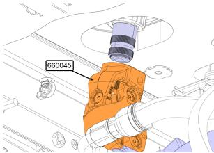
9. Push up the joint and steering column shaft to connect the joint on the steering gearbox.
