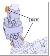
12. Apply torque seal 685353 on each bolts.
