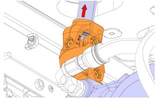
7. Remove the older joint from the steering column shaft and return.
