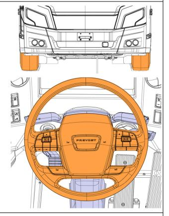
6. Push up the joint and steering column shaft to disconnect the joint from the steering gearbox.
