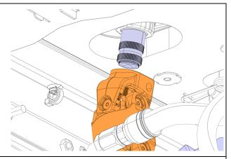
8. Install the new joint 660045 on the steering column shaft.
