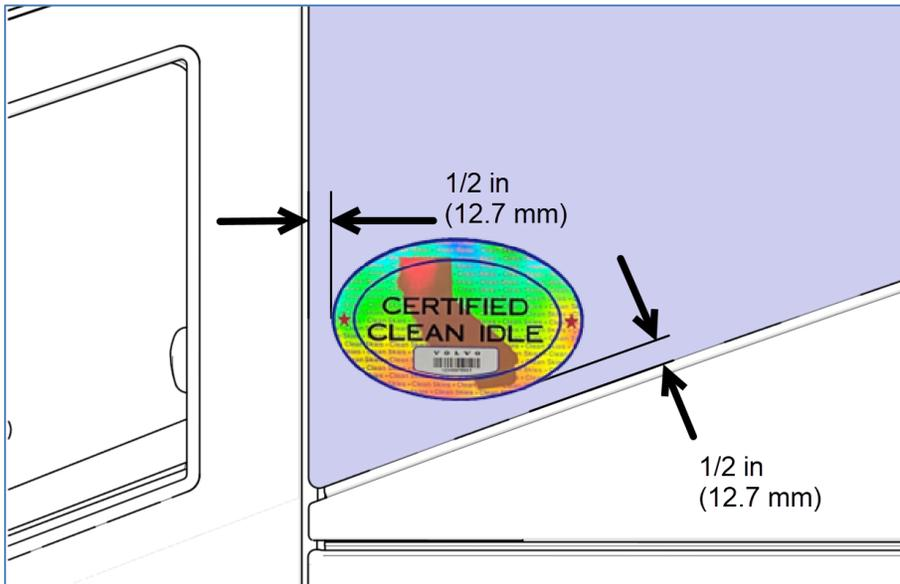
Figure 3: CLEAN IDLE LABEL POSITION ON H3 SERIES
