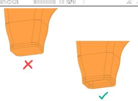
3. Cut the end of the duct at 3/16 inch from the tip using a reciprocating saw.
