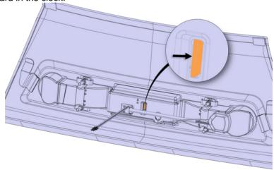
13. Reconnect the Clock connector and reattach the ceiling panel with Velcro in the top.
