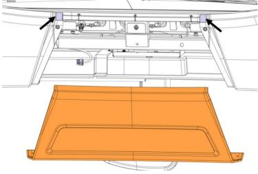
14. Fasten the ceiling panel with the two (2) screws.
