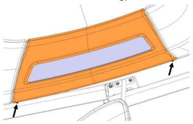
2. Detach the Velcro and remove the central ceiling panel. Disconnect the clock connector.
