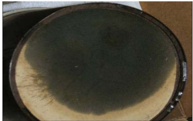
Oil on DPF Filter Inlet or Outlet Surface
