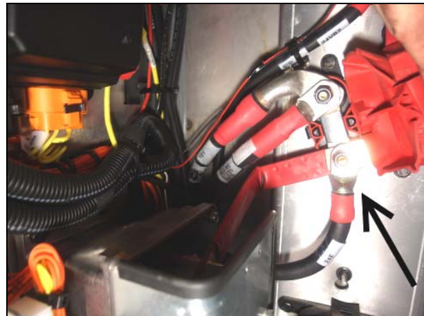
Figure 3: Bussman Junction Block - H3 Series.
