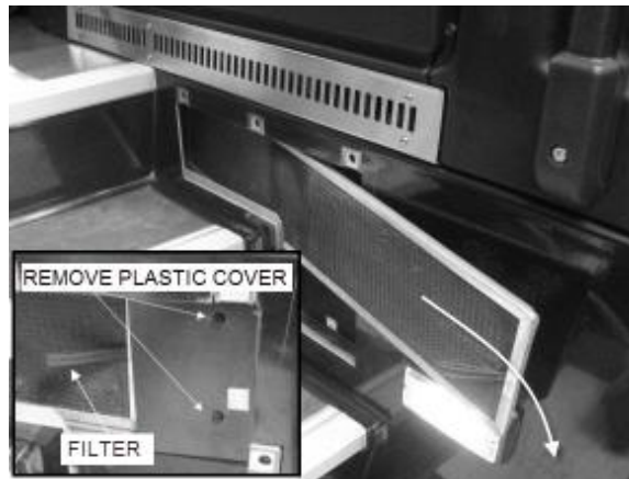
FIGURE 17: REMOVING DRIVER'S SECTION AIR FILTERS
