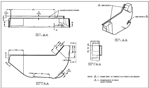
FIGURE 2: OVERHEAD COMPARTMENT COVER
