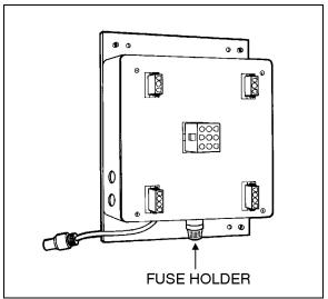
FIGURE 5: PUBLIC ADDRESS SYSTEM CONTROL BOX (PA) 23031
