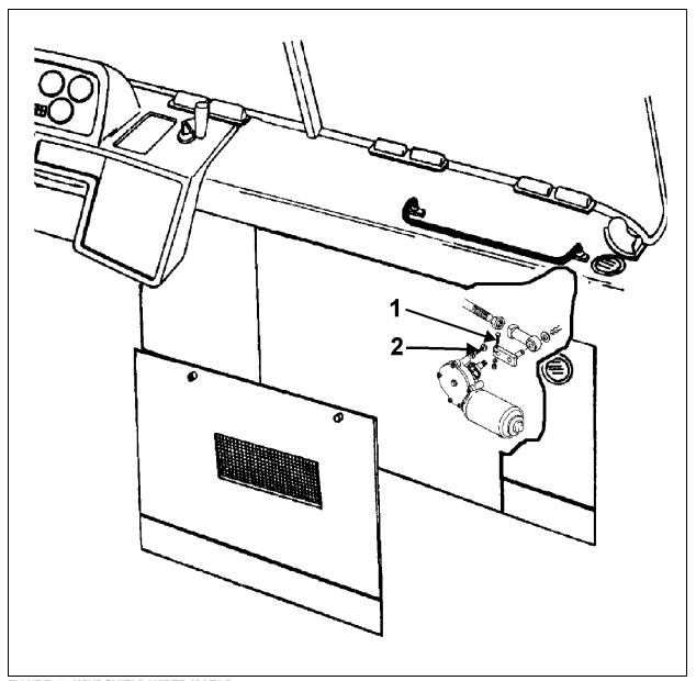
FIGURE 20: WINDSHIELD WIPER MOTOR
