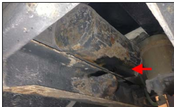
FIGURE 9: APPLICATION DE TECTYL 185GW BLACK
