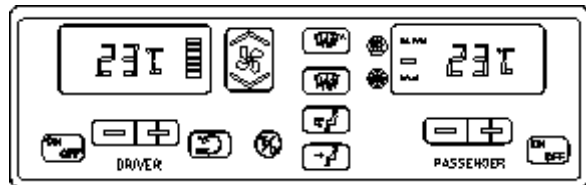
CENTRAL HVAC SYSTEM CONTROL MODULE 22296
