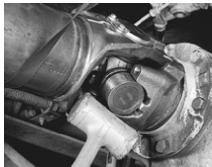
FIGURE 15: UNSEATING BEARING CUP ASSEMBLIES
