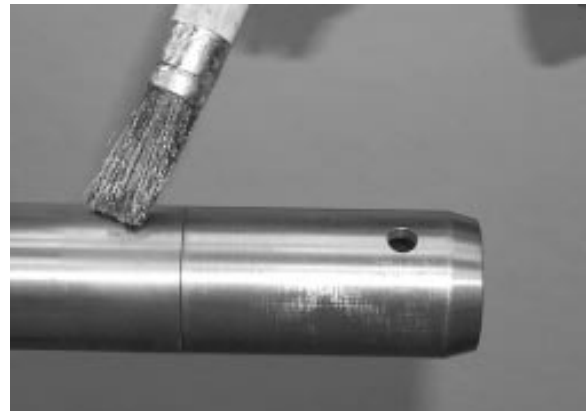
FIGURE 19: APPLY GLEITMO 805 GREASE
