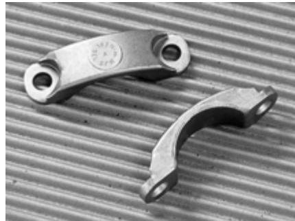
FIGURE 14: COLD FORMED BEARING RETAINERS
