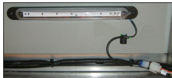
FIGURE 95: BAGGAGE COMPARTMENT LIGHTS LED SEALED UNIT
