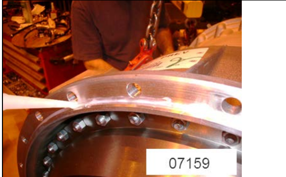
FIGURE 12: SILICONE APPLICATION TRANSMISSION HOUSING
