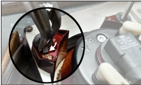
FIGURE 73: UNLOCK THREADED ROD
