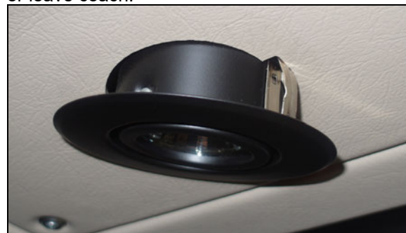
FIGURE 101: DRIVER'S AREA CEILING LIGHT
