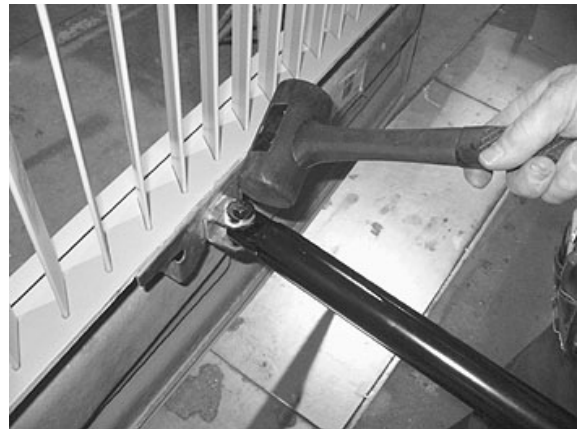
FIGURE 64: DOOR LATERAL ADJUSTMENT
