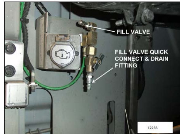
FIGURE 7: REAR VALVE LOCATION (TYPICAL)
