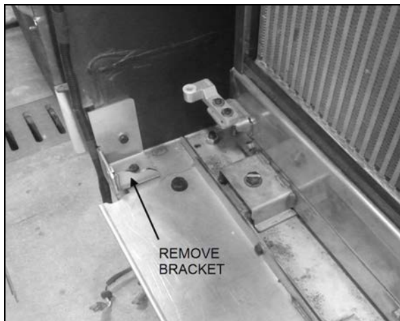
FIGURE 49: RADIATOR DOOR LOWER HINGE BRACKET
