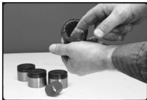
FIGURE 29: GREASING BEARING CUP
