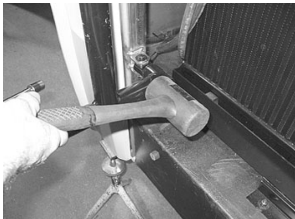
FIGURE 63: PANTOGRAPH ARM ADJUSTMENT
