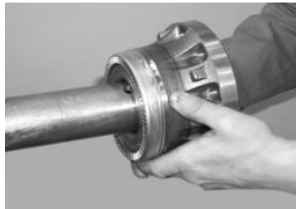
FIGURE 20: SLIDE UNITIZED HUB BEARING OVER SPINDLE
