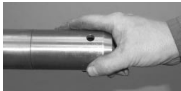
FIGURE 9: INSERTION TOOL PREVOST P/N 491115
