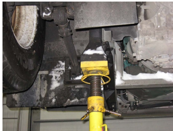
FIGURE 20 : JACK STAND AT CHASSIS HOISTING RECEPTACLE - AFT OF TAG AXLE, CURB SIDE
