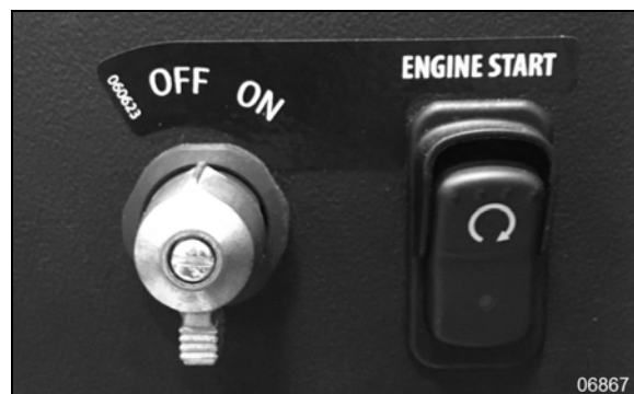
FIGURE 60: SWITCH ARRANGEMENT WITH STARTING MODULE
