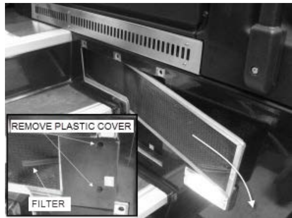
FIGURE 18: REMOVING DRIVER'S SECTION AIR FILTERS
