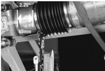
FIGURE 26: POSITION THE END OF THE BOOT AT THE 2.25 INCHES (55-60MM) MARK MADE ON THE YOKE SHAFT SHOULDER
