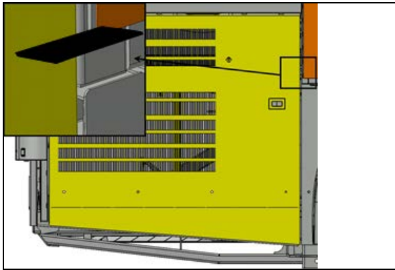
FIGURE 123: USE A RULER (SHOWN IN BLACK) TO CHECK THAT SURFACES ARE EVEN
