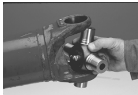
FIGURE 30: POSITION THE JOURNAL CROSS INTO THE YOKE CROSS HOLES WITH THE GREASE ZERK FITTING INWARD TOWARD TUBING
