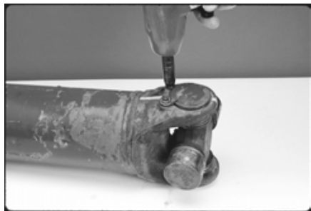
FIGURE 17: SPRING TAB BOLTS REMOVAL
