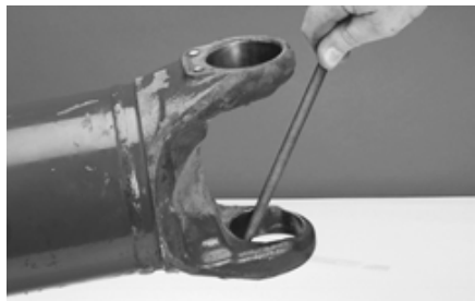
FIGURE 22: RAISED METAL OR FRETTING CAN BE REMOVED FROM YOKE CROSS HOLES WITH A FINE-TOOTHED FILE
