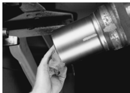
FIGURE 24: CLEAN GREASE FROM SPLINE SLEEVE
