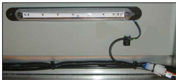
FIGURE 91: BAGGAGE COMPARTMENT LIGHTS LED SEALED UNIT
