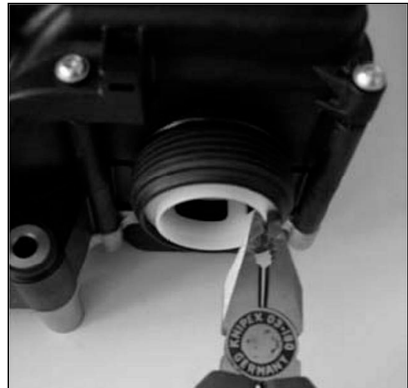
FIGURE 12 : PUMP ASSEMBLY FILTER ELEMENT
