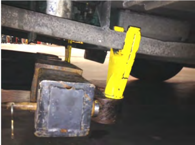
FIGURE 61 : PROPER LOCATION WHEN LIFTING THE SIDE MEMBERS
