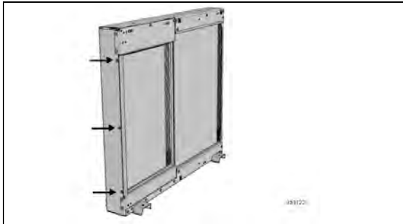
FIGURE 63: CAC LATERAL SUPPORT BOLTS
