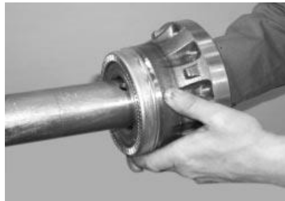
FIGURE 20: SLIDE UNITIZED HUB BEARING OVER SPINDLE
