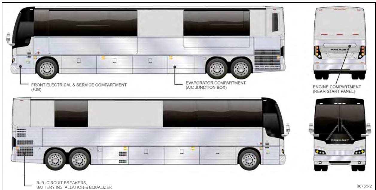
FIGURE 14: ELECTRICAL COMPARTMENTS (X3-45 VIP)
