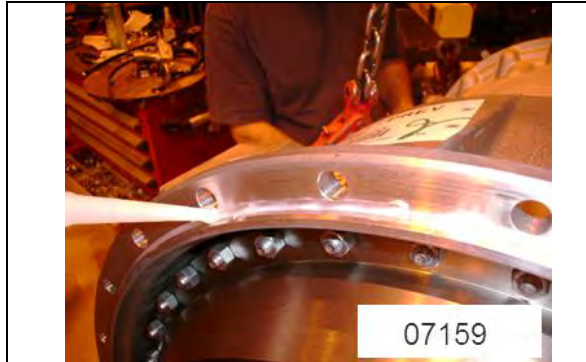
FIGURE 12: SILICONE APPLICATION TRANSMISSION HOUSING
