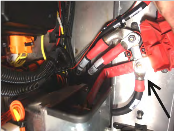
Figure 5: Bussman Junction Block - H3 Series.
