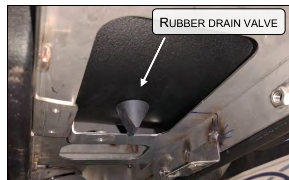
FIGURE 28 RUBBER DRAIN VALVE UNDER FILTER
