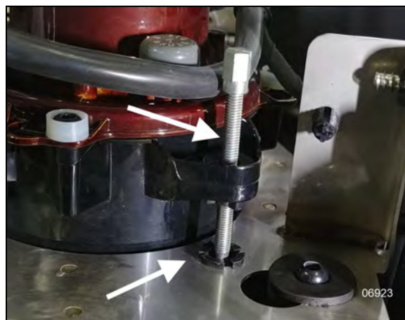
FIGURE 74: UNFASTEN PLASTIC MOUNTS
