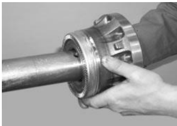
FIGURE 11: SLIP UNITIZED HUB BEARING OVER SPINDLE
