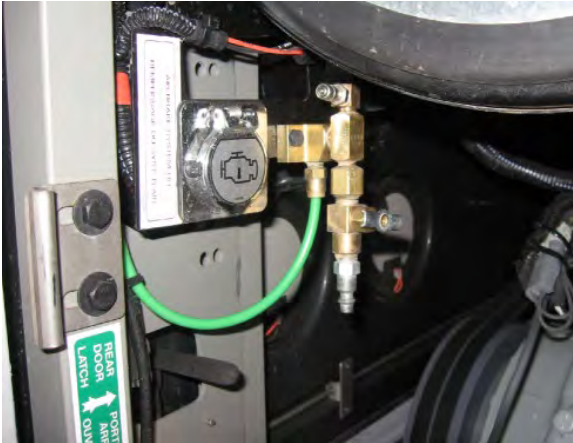
FIGURE 23 : ENGINE COMPARTMENT EMERGENCY AIR-FILL VALVE
