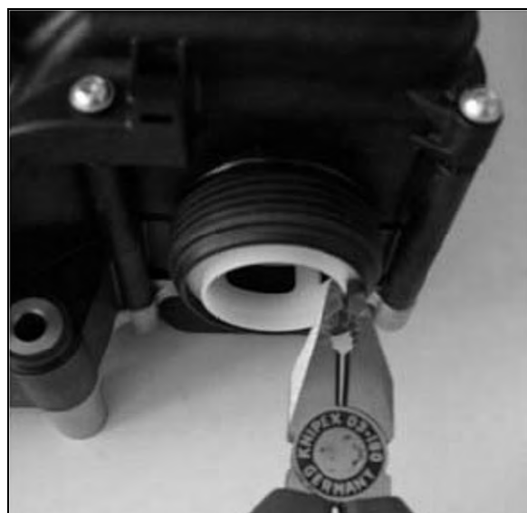
FIGURE 13 : PUMP ASSEMBLY FILTER ELEMENT
