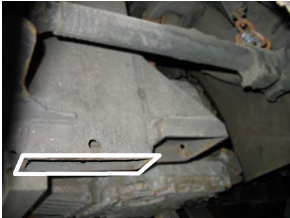
FIGURE 3 : CHASSIS HOISTING POINTS - AFT OF TAG AXLE (BOTH SIDES)
