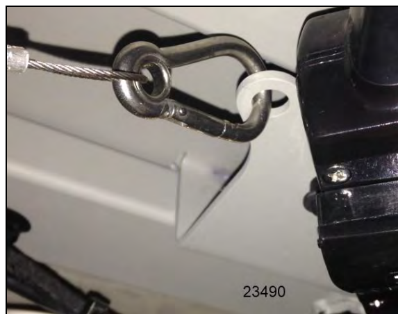
FIGURE 58: PROTECTIVE WIRE INSTALLATION
