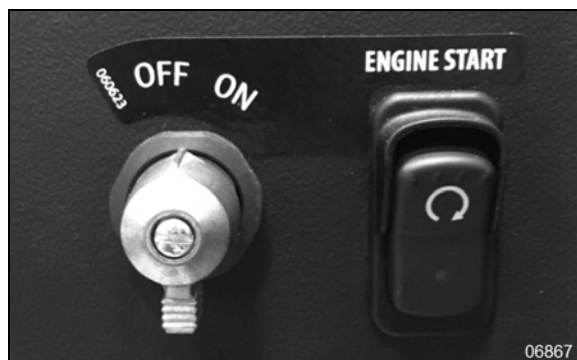
FIGURE 60: SWITCH ARRANGEMENT WITH STARTING MODULE
