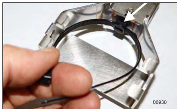
FIGURE 99: CABLE TIE INSTALLATION
