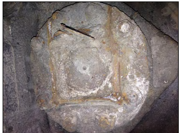
FIGURE 5: HEAVILY CORRODED COACH WITH BROKEN TAG AXLE. THIS IMAGE SHOWS THE SPINDLE MOUNTING PLATE SEPARATED FROM THE REST OF THE TAG AXLE
