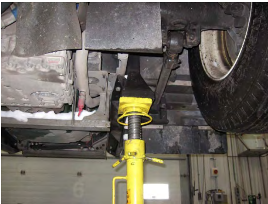
FIGURE 19 : JACK STAND AT CHASSIS HOISTING RECEPTACLE - AFT OF TAG AXLE, ROAD SIDE
