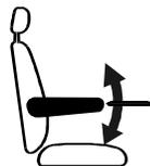
The driver's seat can be equipped with two folding armrests which can be raised or lowered for convenience.
