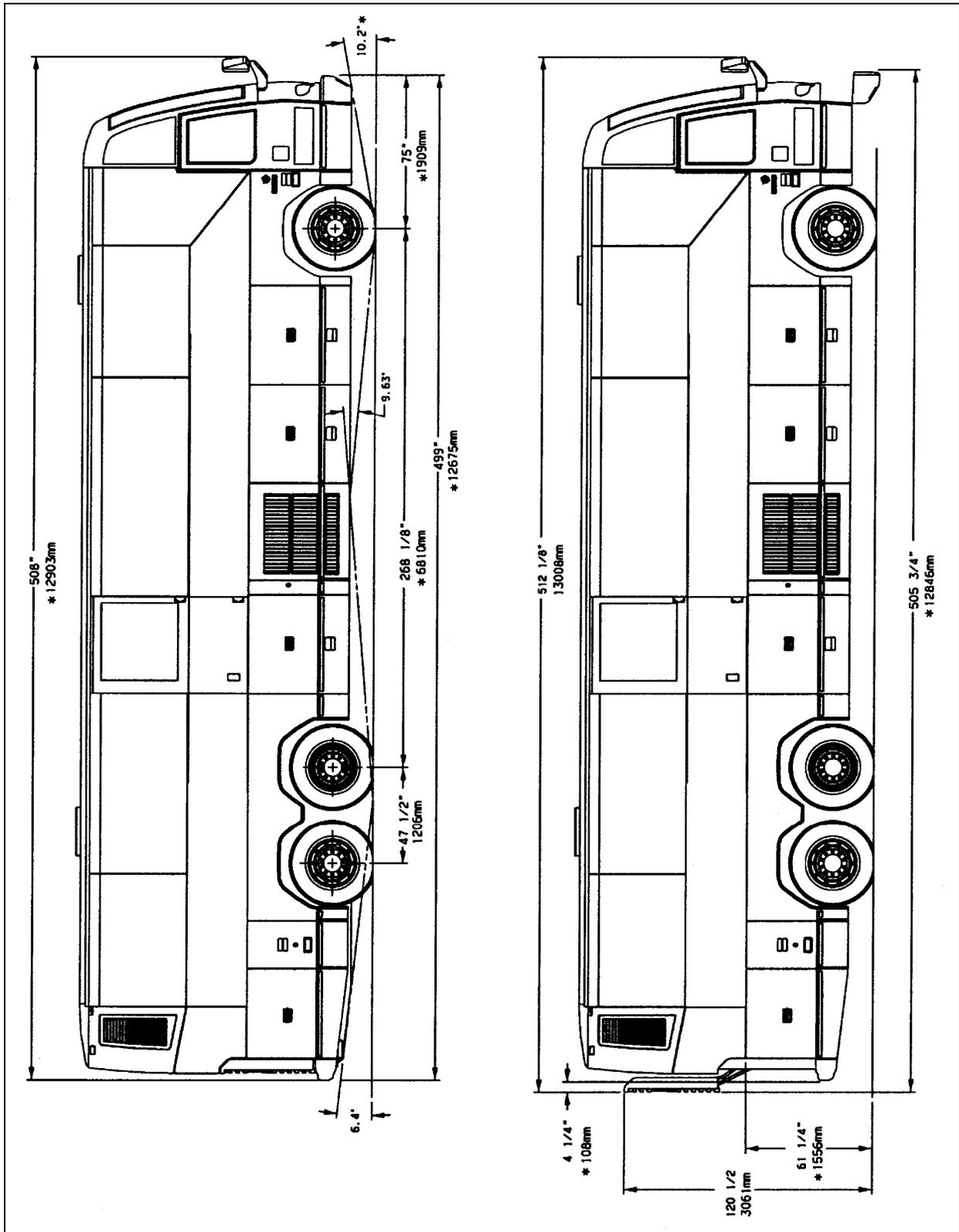
H3-41 OVERALL DIMENSIONS (SIDE ELEVATION)
