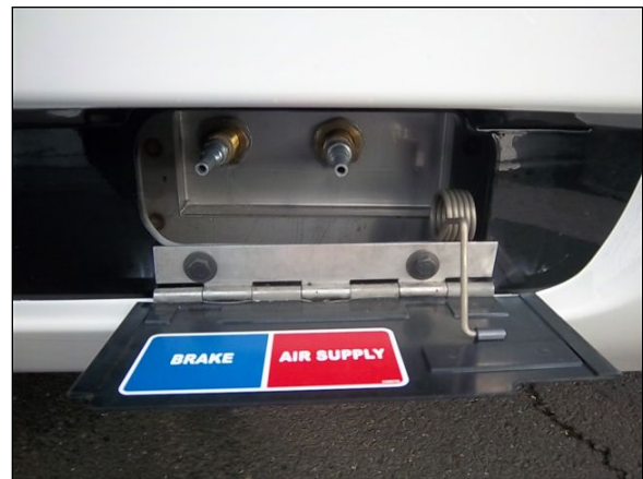
QUICK CONNECTOR FITTINGS ON FRONT BUMPER
