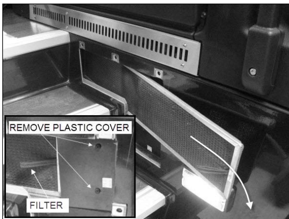
REMOVING DRIVER'S SECTION AIR FILTER
