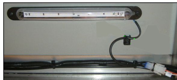
FIGURE 95: BAGGAGE COMPARTMENT LIGHTS LED SEALED UNIT
