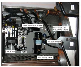
FIGURE 24: CONDENSER COMPARTMENT (A/C)
