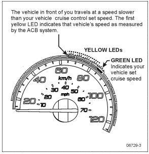
FIGURE 32: EXAMPLE OF THE SPEEDOMETER LED DISPLAY WHEN THE FORWARD VEHICLE IS SLOWER WHILE THE COACH TRAVELS WITH THE ACB CRUISE CONTROL ON AND SET
