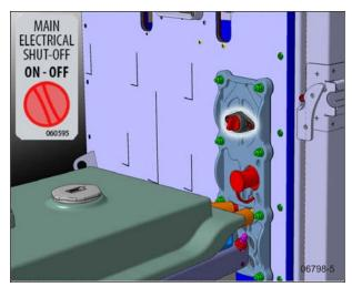
FIGURE 2: MAIN ELECTRICAL SHUT-OFF SWITCH
