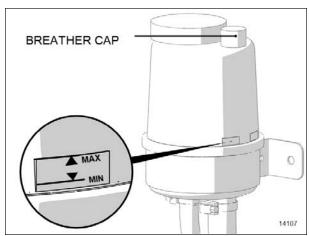
FIGURE 7: POWERSTEERING FLUID TANK
