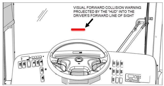
FIGURE 30: HEAD-UP DISPLAY PROJECTED VISUAL WARNING
