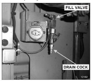
FIGURE 10: ENGINE COMPARTMENT FILL VALVES
