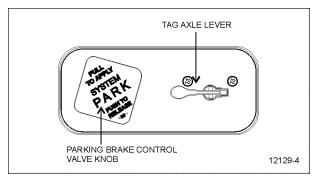
FIGURE 15: TAG AXLE CONTROL VALVE
