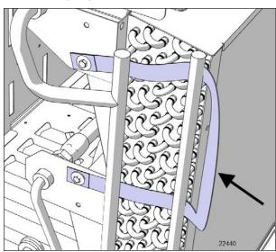
FIGURE 23: CONDENSER CORE STRAP
