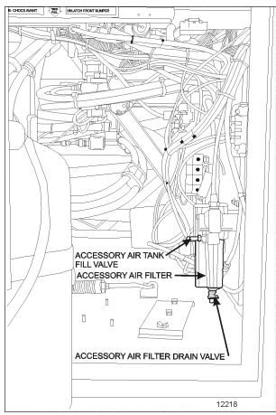
FIGURE 4: FRONT SERVICE COMPARTMENT
