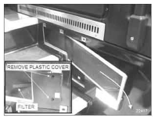
FIGURE 21: REMOVING DRIVER'S SECTION AIR FILTER
