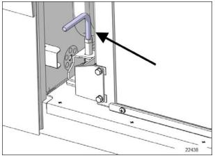
FIGURE 21: BOTTOM CONDENSER UNIT LATCH
