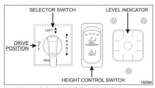
FIGURE 13: LEVEL LOW SYSTEM CONTROLS
