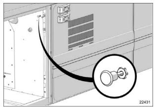
FIGURE 25: EVAPORATOR DOOR RELEASE LATCH
