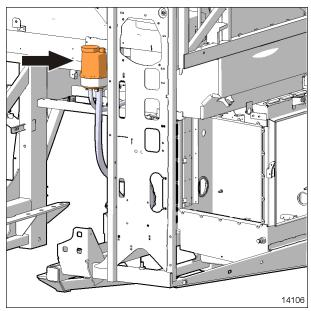
FIGURE 6: POWER STEERING RESERVOIR
