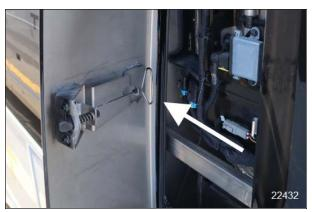
FIGURE 17: SCR ACCESS DOOR HANDLE
