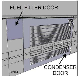
FIGURE 18: CONDENSER COMPARTMENT DOOR (A/C)
