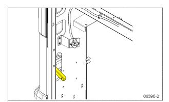
FIGURE 6: ENGINE COMPARTMENT DOOR RELEASE LEVER
