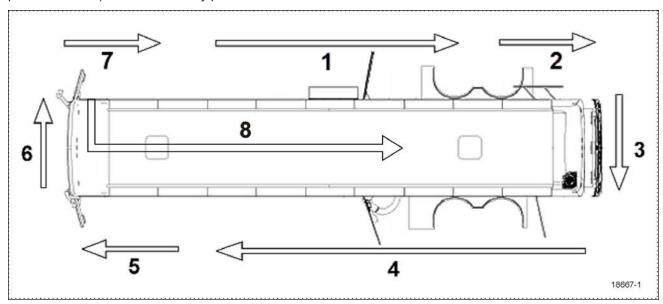
FIGURE 24: X3 SERIES WALK-AROUND INSPECTION
