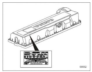
FIGURE 3: VOLVO D13 ENGINE DATA PLATE
