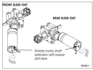
FIGURE 11: SLIDE-OUT MOTOR MANUAL ACTIVATION
