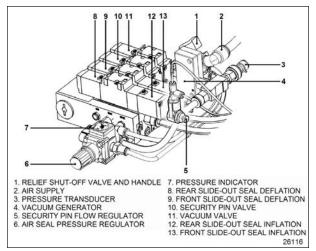
FIGURE 10: PNEUMATIC CONTROL PANEL
