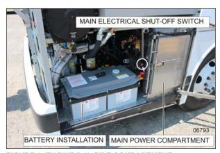
FIGURE 9: ENGINE R.H. SIDE COMPARTMENT (TYPICAL)
