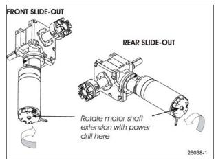
FIGURE 8: SLIDE-OUT MOTOR MANUAL ACTIVATION
