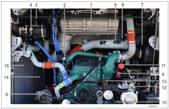
FIGURE 3: ENGINE COMPARTMENT FEATURING VOLVO D13 ENGINE
