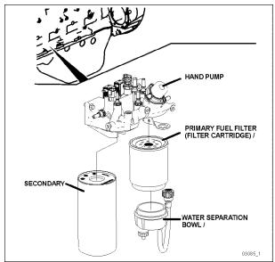
FIGURE 13: FUEL FILTERS WITH VOLVO D13 ENGINE
