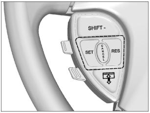
FIGURE 27: CRUISE CONTROL BUTTONS
