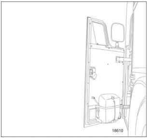
FIGURE 28: FRONT SERVICE COMPARTMENT DOOR
