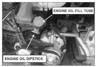
FIGURE 1: ENGINE OIL DIPSTICK - VOLVO D13 ENGINE
