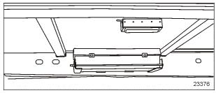
FIGURE 3: WARNING REFLECTORS LOCATION (X3 SERIES)
