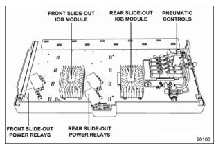
FIGURE 6: SLIDE-OUT CONTROL PANEL
