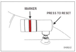
FIGURE 19: AIR FILTER RESTRICTION INDICATOR
