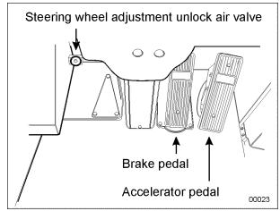
FIGURE 4: FOOT OPERATED CONTROLS
