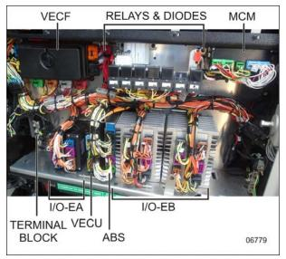
FIGURE 27: FRONT ELECTRICAL COMPARTMENT
