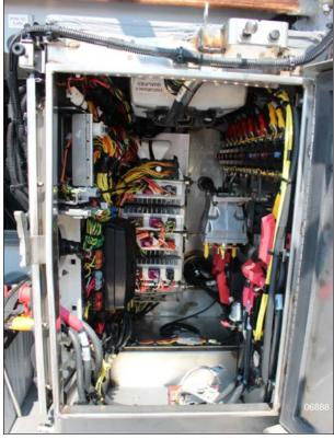
FIGURE 10: MAIN POWER COMPARTMENT (TYPICAL)
