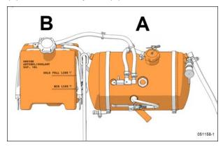
Check the coolant level into the recovery tank (B) when the engine is cold (ambient temperature).
