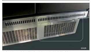
FIGURE 20: DRIVER'S AREA AIR FILTER GRILL REMOVAL
