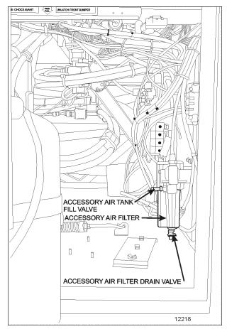
FIGURE 11: FRONT SERVICE COMPARTMENT
