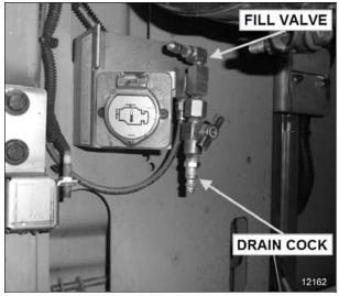
FIGURE 5: FILL FITTING IN ENGINE COMPARTMENT
