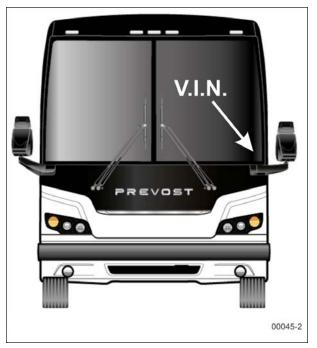
FIGURE 9: VEHICLE IDENTIFICATION NUMBER (X3 SERIES)
