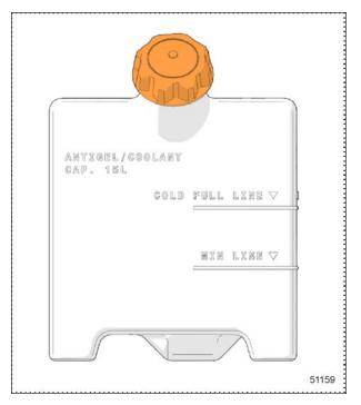
Fill the recovery tank with the same 50/50 waterantifreeze mixture already in the cooling system. Do not mix two different types of coolant. Refer to the Maintenance Manual for proper coolant type specifications or see the label affixed near the coolant surge tank on the vehicle.
