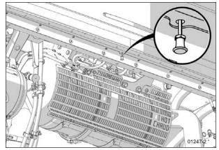
FIGURE 8: AFTERTREATMENT ACCESS DOOR LATCH
