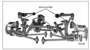
FIGURE 6: INDEPENDENT FRONT SUSPENSION
