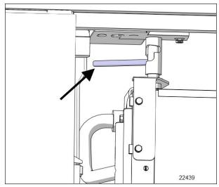
FIGURE 22: TOP CONDENSER UNIT LATCH
