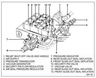
FIGURE 7: PNEUMATIC CONTROL PANEL
