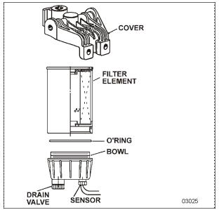
FIGURE 12: FUEL FILTER/WATER SEPARATOR
