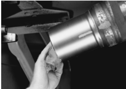
FIGURE 22: CLEAN GREASE FROM SPLINE SLEEVE
