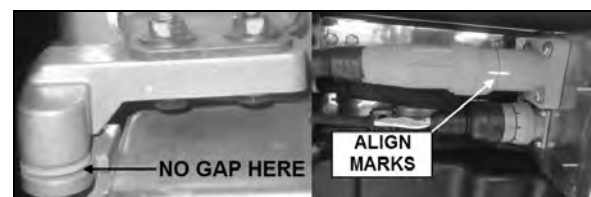
FIGURE 26: INSTALLED HINGE &amp; MAIN CONNECTOR
