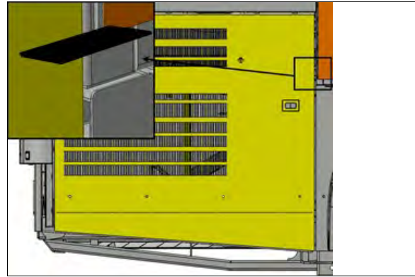
FIGURE 132: USE A RULER (SHOWN IN BLACK) TO CHECK THAT SURFACES ARE EVEN
