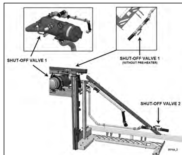
FIGURE 28: HEATER SHUT-OFF VALVES POSITION
