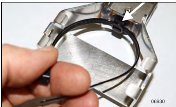
FIGURE 107: CABLE TIE INSTALLATION
