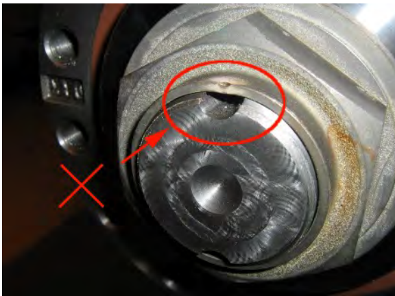
FIGURE 27: LIP INADEQUATELY PRESSED IN – REJECTED
