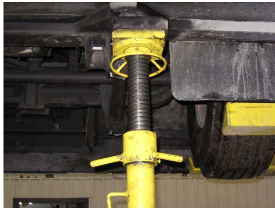
FIGURE 18 : JACK STAND AT CHASSIS HOISTING RECEPTACLE - AFT OF FRONT AXLE, CURB SIDE
