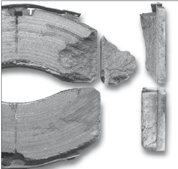
FIGURE 26: MAJOR BREAKOUTS ON THE SURFACE OF THE BRAKE PAD ARE NOT PERMITTED
