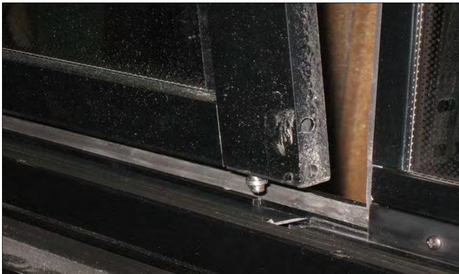
FIGURE 108: DISENGAGING THE BOTTOM OF THE SASH
