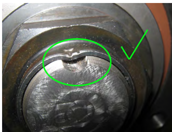
FIGURE 24: CORRECT - PREVENTS THE NUT FROM GETTING LOOSE
