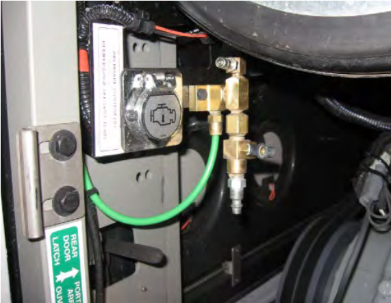
FIGURE 23 : ENGINE COMPARTMENT EMERGENCY AIR-FILL VALVE
