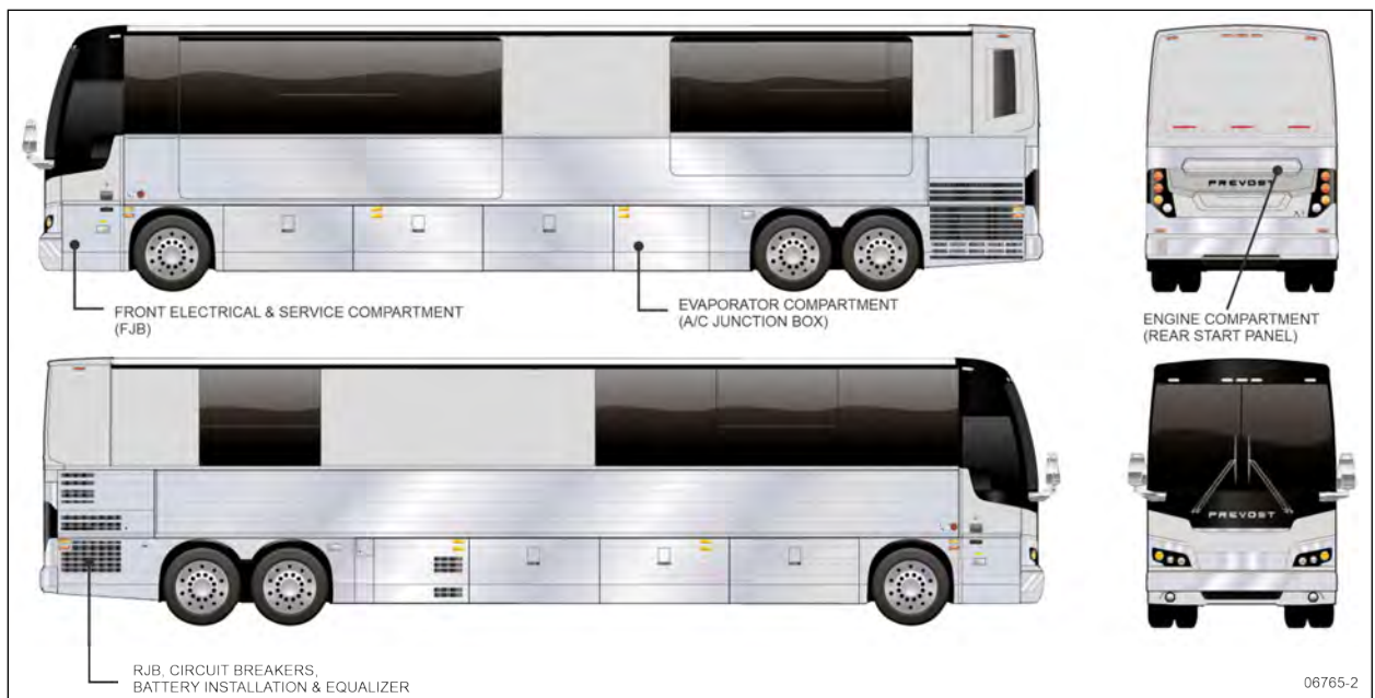
FIGURE 15: ELECTRICAL COMPARTMENTS (X3-45 VIP)
