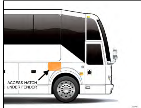
FIGURE 66: ACCESS TO LEVELING SCREWS, FORE
