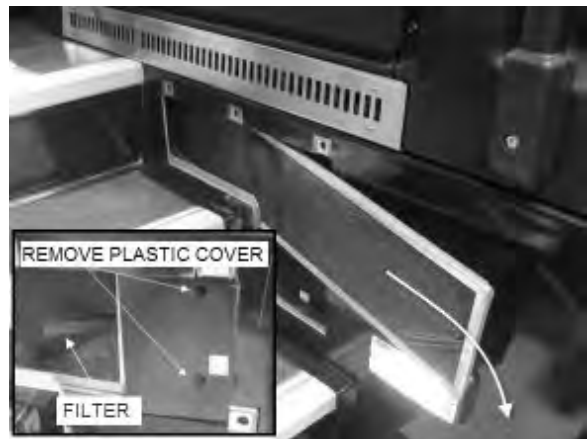
FIGURE 18: REMOVING DRIVER'S SECTION AIR FILTERS
