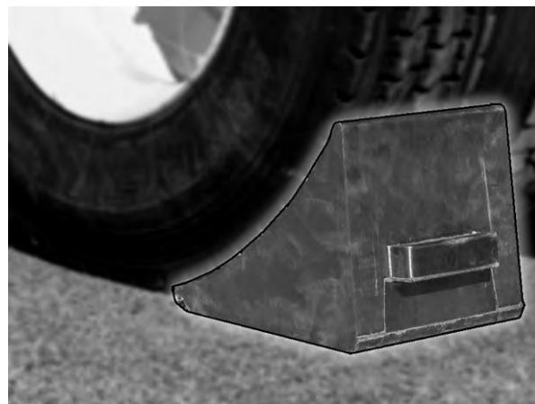
FIGURE 21 CHOCK THE FRONT AND REAR WHEELS
