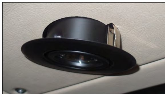
FIGURE 118: DRIVER'S AREA CEILING LIGHT
