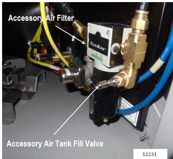
FIGURE 4: FRONT SERVICE COMPARTMENT
