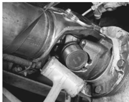
FIGURE 13: UNSEATING BEARING CUP ASSEMBLIES
