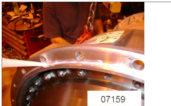
FIGURE 12: SILICONE APPLICATION TRANSMISSION HOUSING
