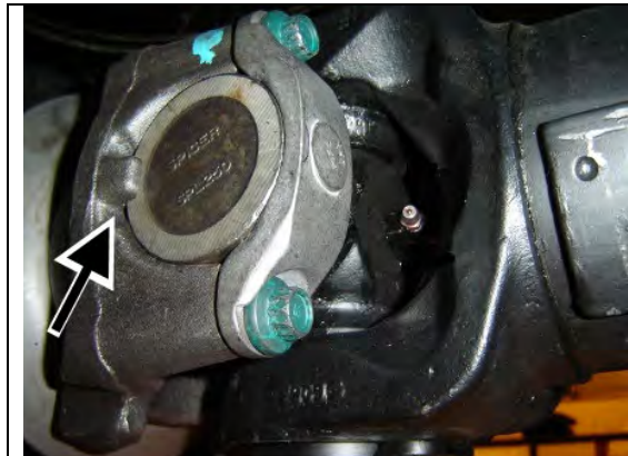
FIGURE 26: YOKE TAB (EAR)
