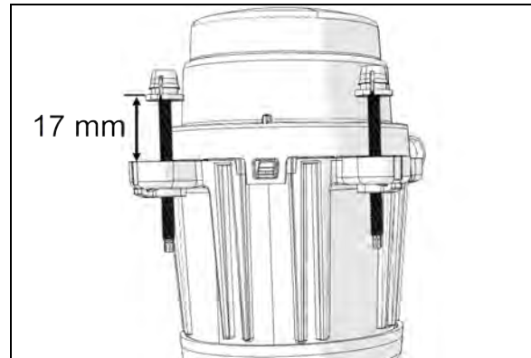
FIGURE 63: LOW BEAM LED MODULE
