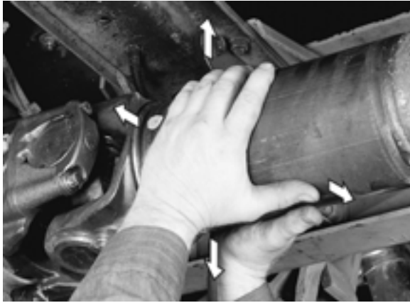
FIGURE 6: CHECK FOR LOOSENESS
