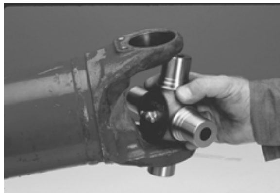
FIGURE 28: POSITION THE JOURNAL CROSS INTO THE YOKES CROSS HOLES WITH THE GREASE ZERK FITTING INWARD TOWARD TUBING
