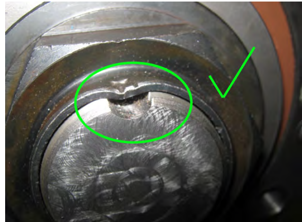
FIGURE 23: CORRECT - PREVENTS THE NUT FROM GETTING LOOSE
