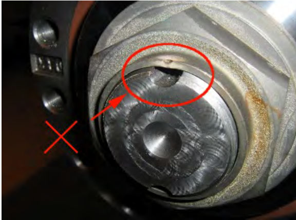
FIGURE 26: LIP INADEQUATELY PRESSED IN – REJECTED
