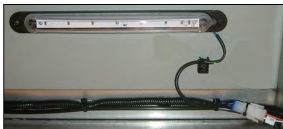
FIGURE 77: BAGGAGE COMPARTMENT LIGHTS LED SEALED UNIT
