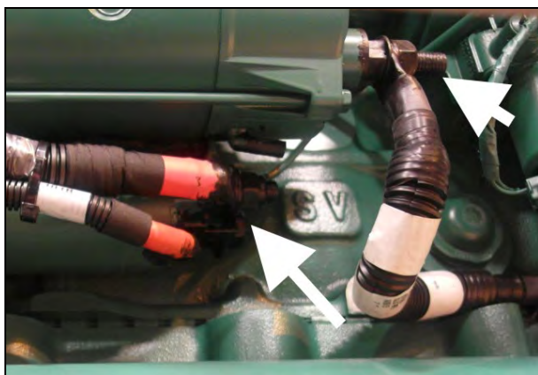
Figure 30: Starter power cable and ground cable lugs protected with Color Guard rubber coating.
