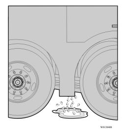
Water spilled from the vent valve.
