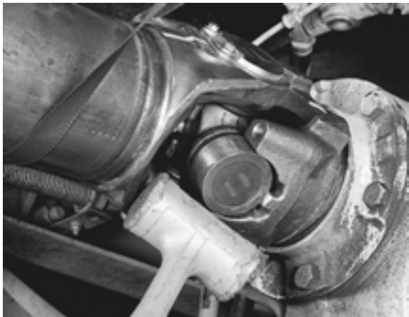
FIGURE 13: UNSEATING BEARING CUP ASSEMBLIES
