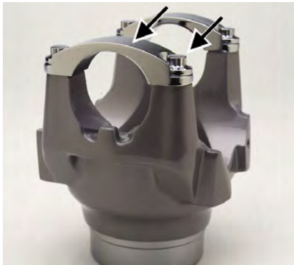
FIGURE 2: COLD FORMED BEARING RETAINER AND BOLTS AS USED ON PREVOST X3-45 COMMUTER
