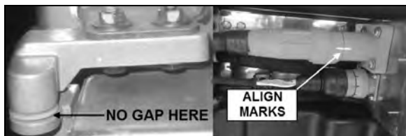
FIGURE 27: INSTALLED HINGE & MAIN CONNECTOR
