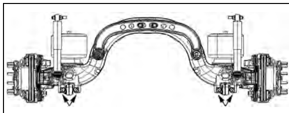
FIGURE 5: JACKING POINTS ON TAG AXLE 11023
