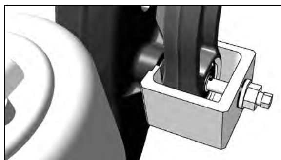
FIGURE 6: INSTALLING EXTRACTOR TOOL
