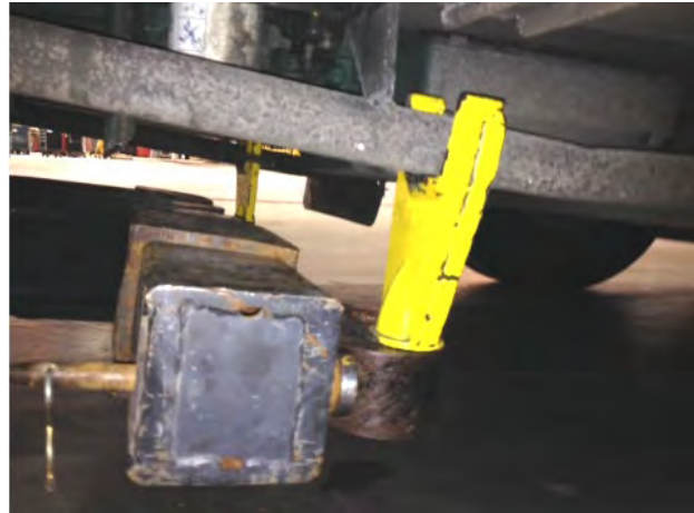
Figure 68: PROPER LOCATION WHEN LIFTING THE SIDE-MEMBERS
