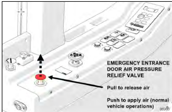
FIGURE 50: AIR PRESSURE RELIEF VALVE ON THE LATERAL
