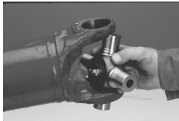
FIGURE 28: POSITION THE JOURNAL CROSS INTO THE YOKE CROSS HOLES WITH THE GREASE ZERK FITTING INWARD TOWARD TUBING
