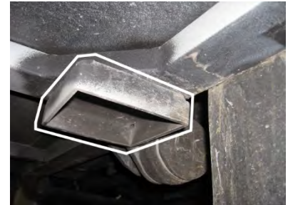
FIGURE 4: CHASSIS HOISTING RECEPTACLES - AFT OF FRONT AXLE
