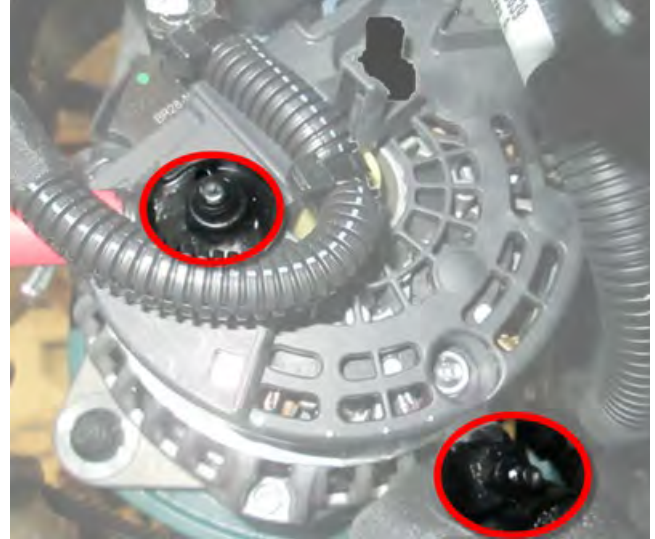
Figure 28: Lower R.H. side Bosch alternator power cable lug protected with Color Guard rubber coating.
