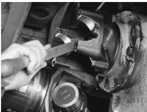
FIGURE 14: RAISED METAL OR FRETTING ON OPEN YOKE CROSS HOLES
