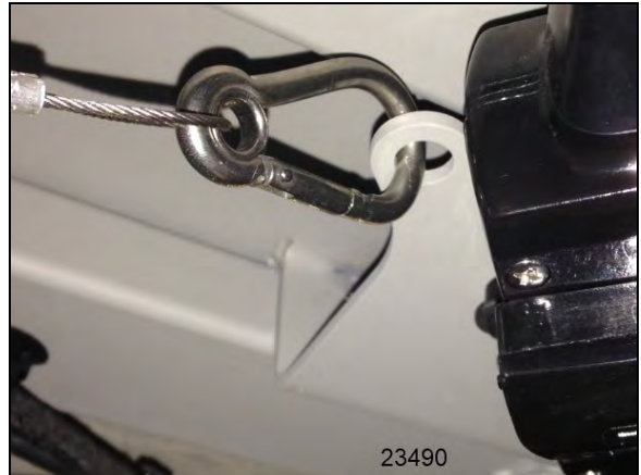
FIGURE 21: PROTECTIVE WIRE INSTALLATION
