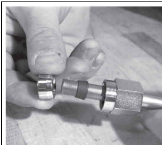
FIGURE 15: PLACE A NUT, FERRULE AND SLEEVE ONTO TUBING
