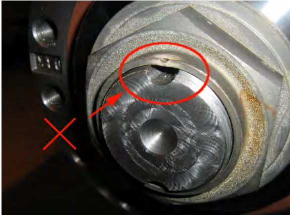
FIGURE 26: LIP INADEQUATELY PRESSED IN – REJECTED
