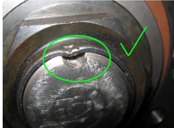
FIGURE 23: CORRECT - PREVENTS THE NUT FROM GETTING LOOSE
