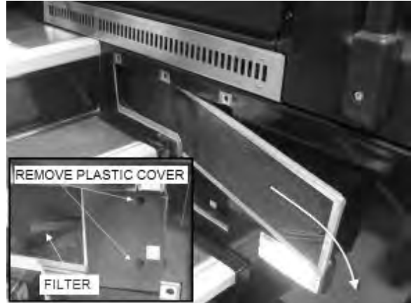
FIGURE 9: REMOVING DRIVER'S SECTION AIR FILTERS
