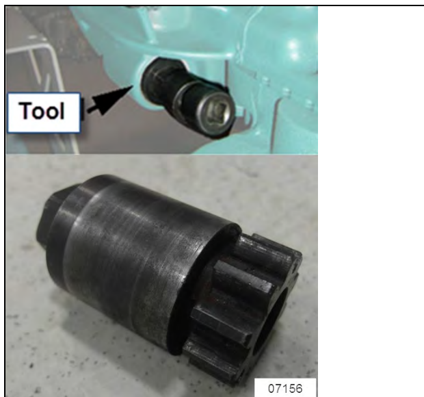
FIGURE 10: VOLVO ENGINE TURNING TOOL #88800014
