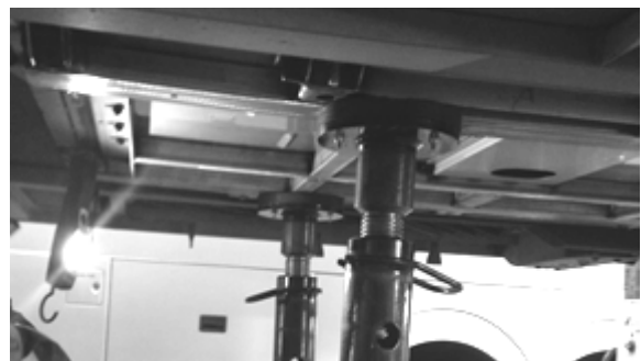
FIGURE 21: JACK STANDS UNDER THE FUEL TANK CRADLE
