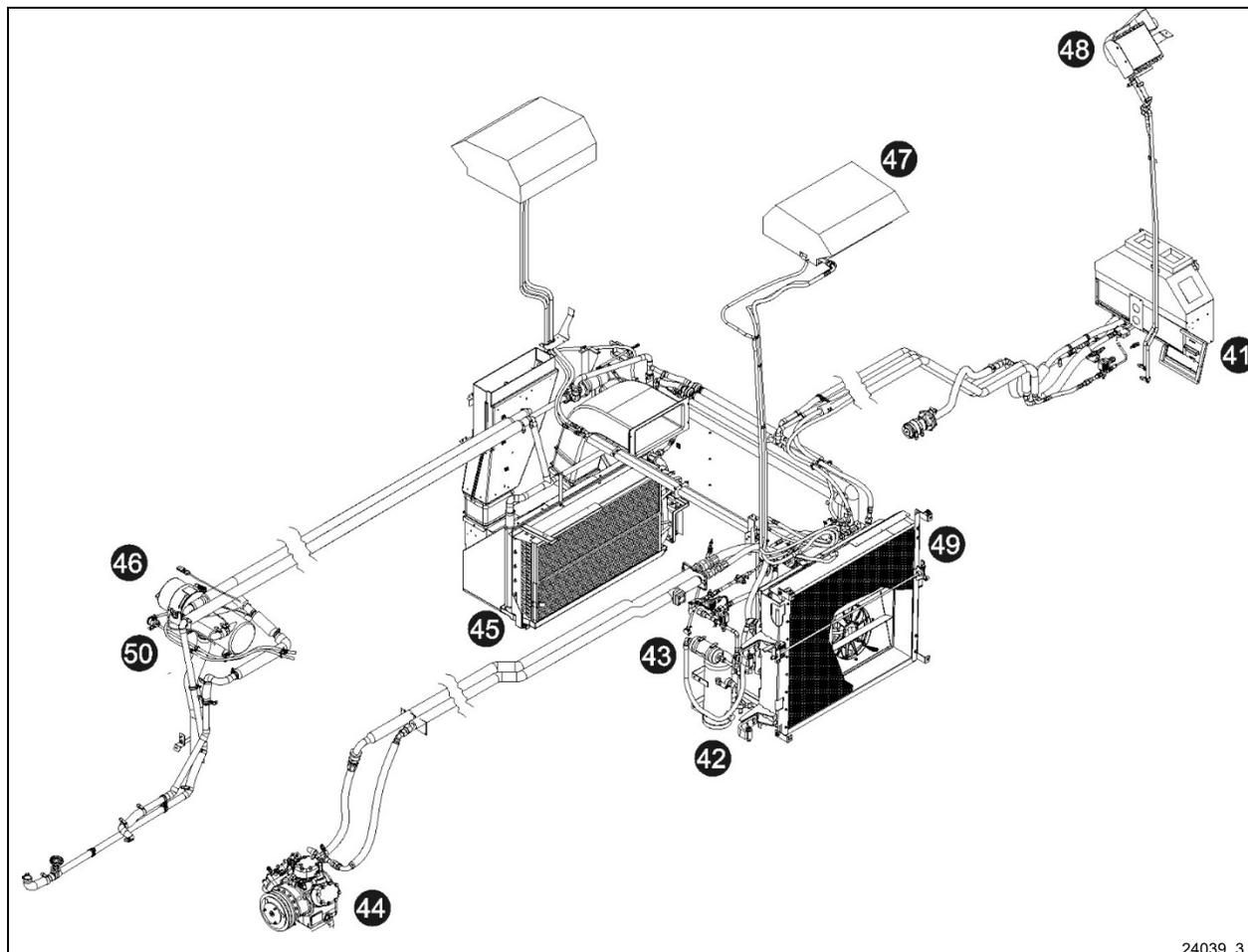
FIGURE 3: LUBRICATION AND SERVICING POINTS – HVAC UNIT
