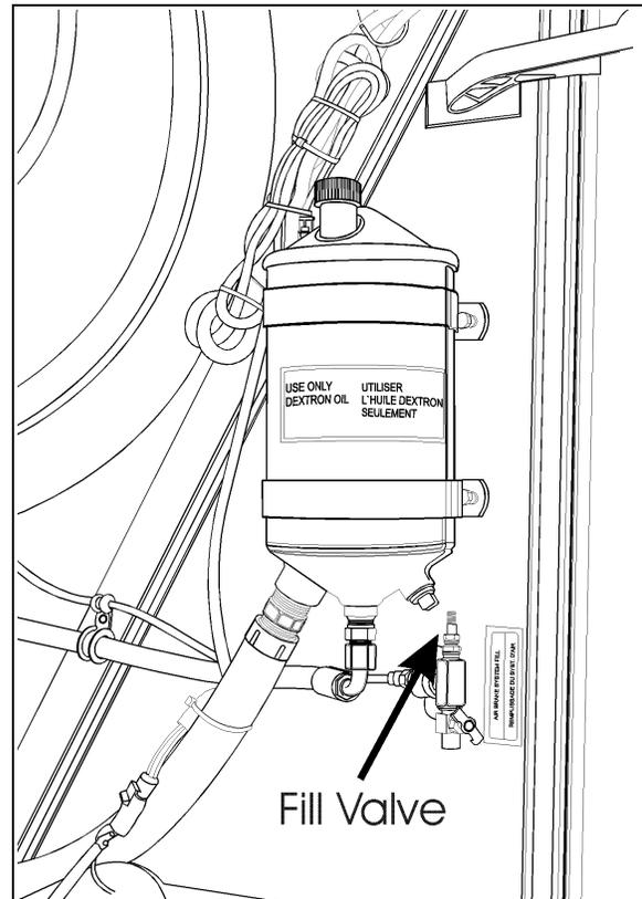
FILL VALVE IN ENGINE COMPARTMENT 12162
