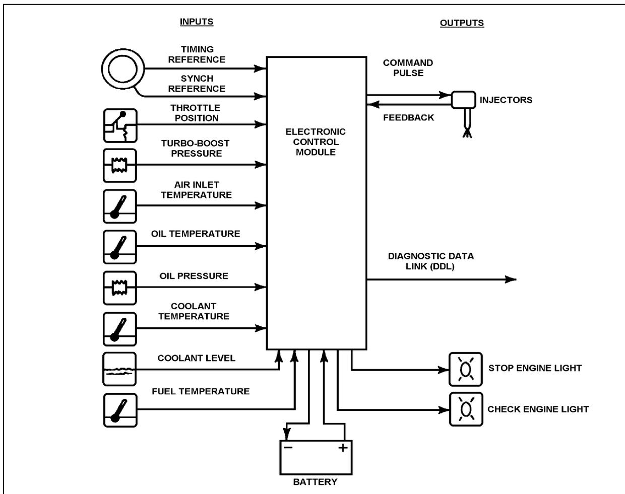
SHEMATIC DIAGRAM OF DDEC IV SYSTEM
