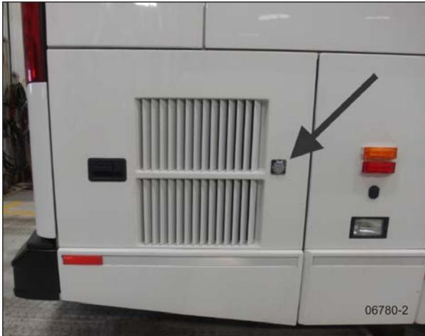
FIGURE 28: BATTERY CHARGER 120-VOLT CONNECTOR – H3
