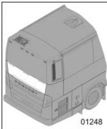
The engine door must be opened before opening the DPF access door. To open the DPF access door, press the latch release lever. Using both hands, push the door up until it locks in place.
