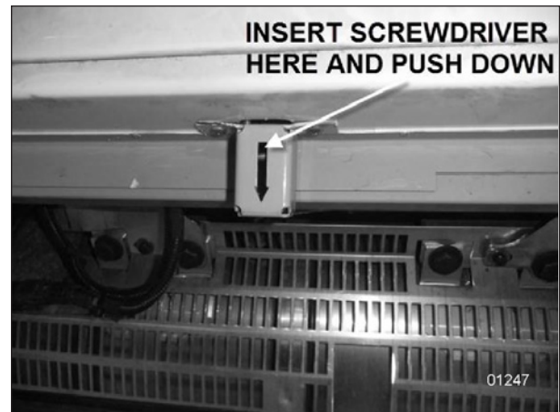
AFTERTREATMENT ACCESS DOOR LATCH
