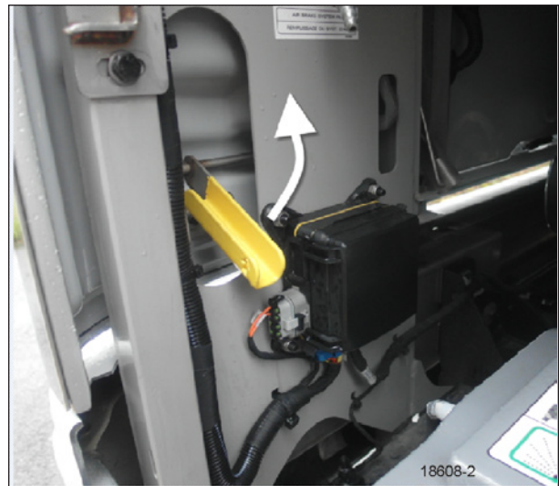
OPENING ENGINE COMPARTMENT REAR DOOR
