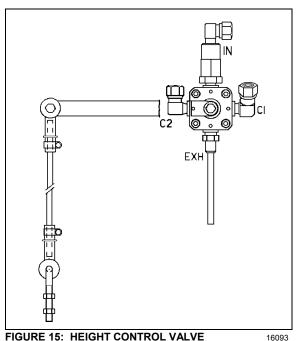
The height control valves automatically add air to, or release air from air springs to maintain constant suspension height regardless of load, or load distribution. Each valve adjusts independently according to the following conditions:
