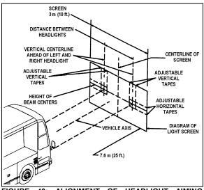
FIGURE 40: ALIGNMENT OF HEADLIGHT AIMING SCREEN 06502
