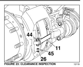
Measure pad to rotor clearance:
