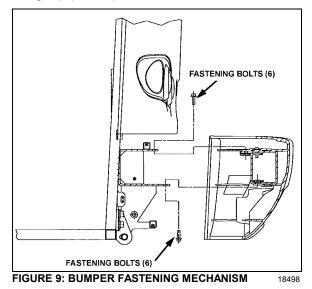
To install molded front bumper, reverse the procedure.
