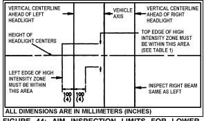
FIGURE 44: AIM INSPECTION LIMITS FOR LOWER-BEAM HEADLIGHTS 06506
