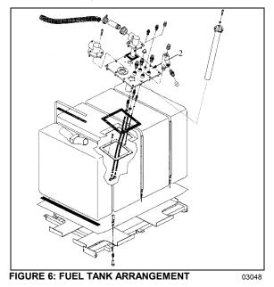
Warning: Before removing the bolts securing the tank support to the frame, make sure the tank is supported adequately. Failure to do so could result in injury as well as damage to the tank.
