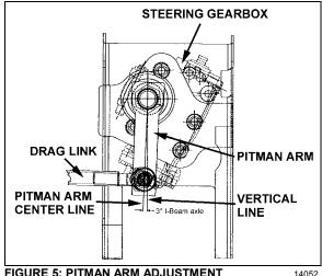
FIGURE 5: PITMAN ARM ADJUSTMENT
