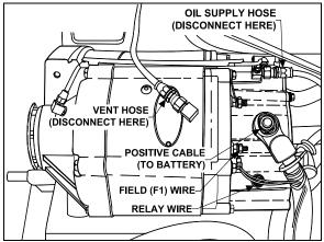
FIGURE 20: ALTERNATOR (HOSES AND WIRES) 06073
