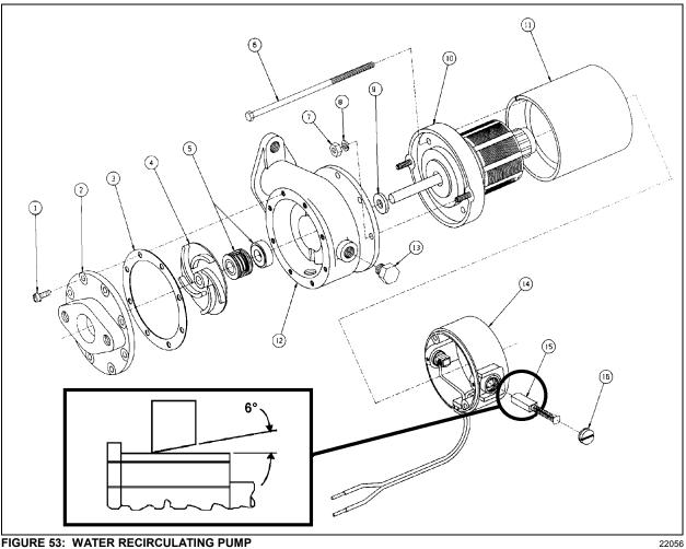
FIGURE 53: WATER RECIRCULATING PUMP
