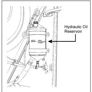
FIGURE 7: HYDRAULIC FLUID RESERVOIR LOCATION 14043
