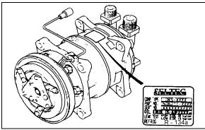
FIGURE 38: COMPRESSOR OIL LABEL
