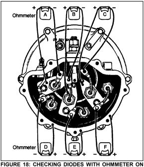
A TYPICAL OIL COOLED ALTERNATOR (END COVER REMOVED) 06071
