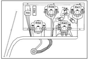
FIGURE 8: CONTROL PANEL IN HVAC COMPARTMENT<sub>06483</sub> Each relay or resistor is identified to facilitate its location (Fig. 9).
