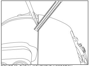
FIGURE 28: RADIAL MOVEMENT INSPECTION
