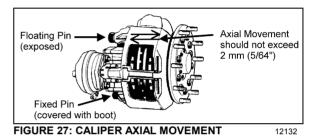
The caliper flotation consists of two pins. One pin (fixed pin) floats and should have minimal movement in the radial direction. The other pin is floating in a rubber bushing. The maximum radial movement should not exceed 2.0 mm (0.080"). To check the radial movement, insert a pry tool between the caliper and carrier near the middle and then measure the relative movement as shown in figure 28.
