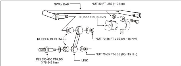
A sway bar is provided on the front and drive axles to increase vehicle stability. It controls lateral motion
