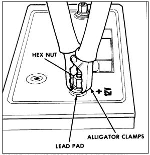
FIGURE 12: ALLIGATOR CLAMPS AND BATTERY 06065
