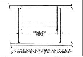
FIGURE 47: PANTOGRAPH DOOR ADJUSTMENT 18063
