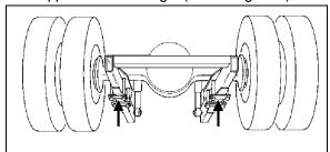
FIGURE 5: JACKING POINTS ON DRIVE AXLE H3B762
