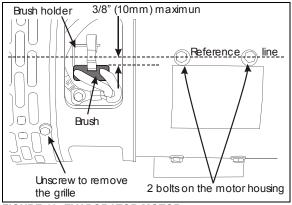
FIGURE 18: EVAPORATOR MOTOR
