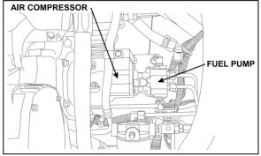
FIGURE 8: AIR COMPRESSOR INSTALLATION 03053
