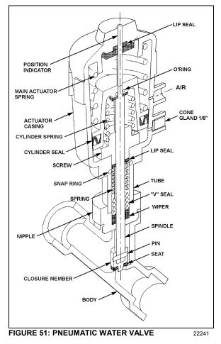
12.8.3 Pneumatic Water Valve Reassembly
