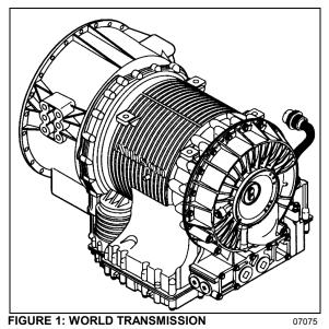
Gear selection and torque converter modes are controlled by a microcomputer-based electronic transmission management system. It is fed information regarding throttle position, operator range selection, engine speed, turbine speed, transmission output speed and various system pressures from special electronic sensors.
