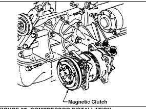
FIGURE 37: COMPRESSOR INSTALLATION
