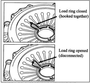
FIGURE 8: RELEASE BEARING RETAINING CLIP 07081
