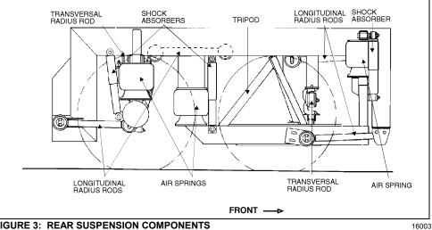
FIGURE 3: REAR SUSPENSION COMPONENTS
