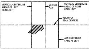
FIGURE 42: HIGH-INTENSITY ZONE (SHADED AREA) OF A PROPERLY AIMED LOWER BEAM ON THE AIMING SCREEN 7.6 M (25 FT) ON FRONT OF VEHICLE 06504  The inspection limits for high-beam headlights shall be with the center of the high-intensity zone from 10 cm (4 in) up to 10 cm (4 in) down; and, from 10 cm (4 in) left to 10 cm (4 in) right on a screen at 7.6 m (25 ft.) (Fig. 44).
