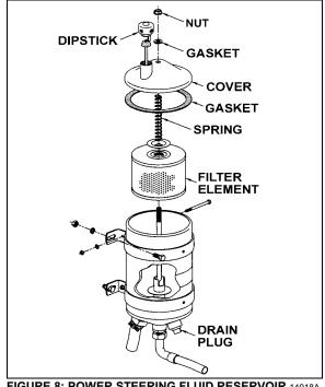
FIGURE 8: POWER STEERING FLUID RESERVOIR 14018A
