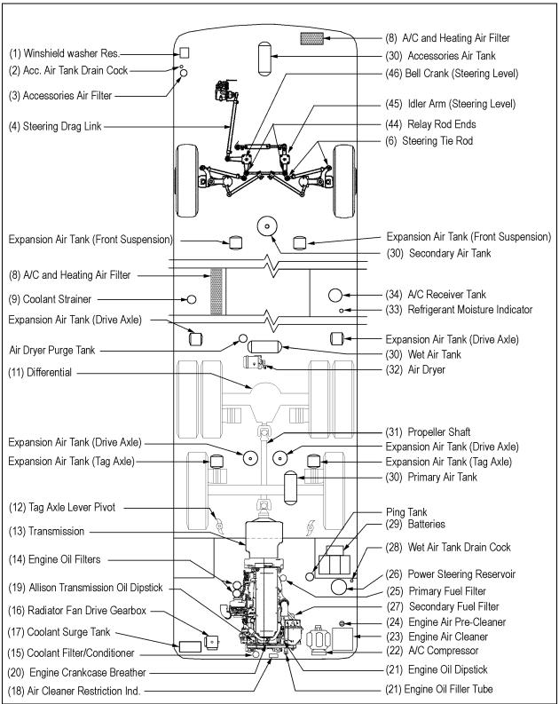
FIGURE 3: LUBRICATION AND SERVICING POINTS ON INDEPENDENT FRONT SUSPENSION VEHICLES (TYPICAL) 24005
