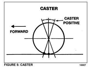
Excessive caster results in hard steering around corners. A shimmy may also develop when returning to the straight ahead position (pulling out of curves).
