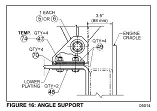
Center seat assembly in the fan shroud using the horizontal displacement of the fan driving mechanism support. Center with the slots in the floor at anchoring angle support (on some vehicles only). Vertical displacement of the fan clutch is made possible by slots at the base of the fan clutch (on some vehicles only) or by shimming with additional spacers at anchoring locations. Temporarily secure assembly with two nuts (P/N 500709), (74, Fig. 16) at both anchoring locations.
