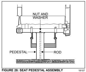
Note: Bottom end of rod is coated with Locktite and threaded in a steel block which slides in the floor track. Removal of rod is possible if loosened from block. Otherwise, slide rod and block assembly to the front end of track after removing all seats located in front.
