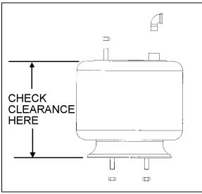
FIGURE 28: TYPICAL AIR SPRING CLEARANCE 16058
