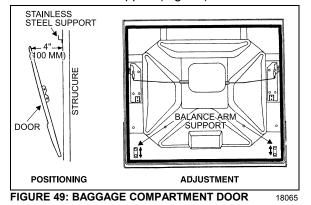
Fully open the door, loosen the two bolts 3. retaining each gas cylinder support to structure, position door parallel with adjacent doors and complete tightening bolts. A measure of 6"  $\pm \frac{1}{4}$ " (150mm  $\pm$  7mm) between door panel lip (at level of upper edge of lower section) and the lateral panel is given as a guide.
