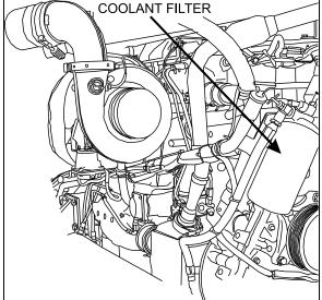
FIGURE 8: COOLANT FILTER
