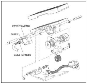
FIGURE 14: ELECTRONIC FOOT PEDAL ASSEMBLY 03035
