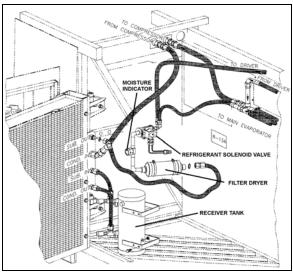
FIGURE 28: A/C CONDENSER COMPARTMENT 22219
