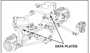
FIGURE 6: ISS TYPICAL SERIAL & MODEL NUMBERS00025C
