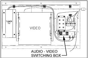
FIGURE 13: INSTALLATION IN PARCEL COMPARTMENT
