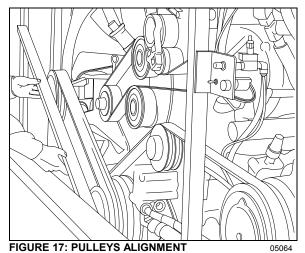
4. Using a universal protractor, check 3"V" pulley's vertical angle with that of engine pulleys. If angles do not correspond, raise
