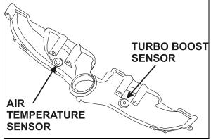
FIGURE 5: TURBO BOOST PRESSURE SENSOR 01023
