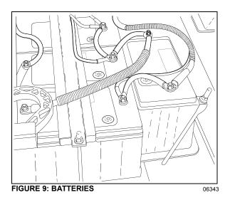
With special cables properly attached to batteries, the metal surfaces that carry the current are completely sealed from the atmosphere. This prevents terminal oxidation and corrosion that may cause starting and charging problems. If new cables are required, sealed terminal cable replacements should be used to retain the reliability of the original maintenancefree connections.
