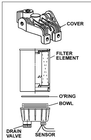
FIGURE 3: FUEL FILTER/WATER SEPARATOR 03025
