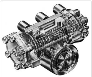
FIGURE 2: POWER STEERING GEAR
