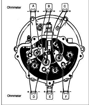
FIGURE 17: CHECKING DIODES WITH OHMMETER ON A TYPICAL OIL COOLED ALTERNATOR (END COVER REMOVED) 06070
