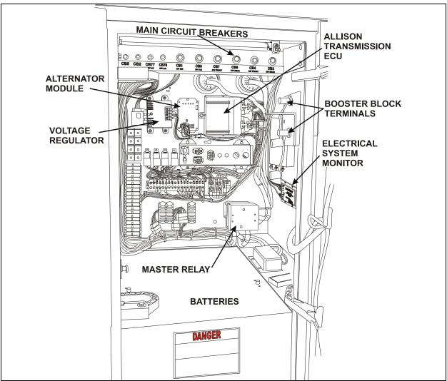
FIGURE 5: MAIN POWER COMPARTMENT
