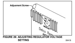
**Note**: If regulator voltage cannot be adjusted to the specified setting, remove the regulator and repair or replace it as necessary.
