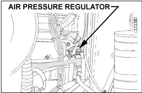
FIGURE 13: AIR PRESSURE REGULATOR (TYPICAL)07037
