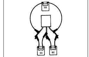
FIGURE 29: CHECKING TRANSISTORS TR2
