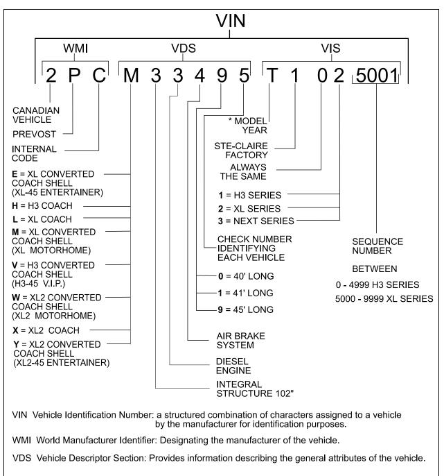
VIS Vehicle Indicator Section: Combination of characters assigned by the manufacturer to distinguish one vehicle from another.
