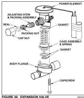
The remote bulb and power assembly is a closed system. The pressure within the remote bulb and power assembly corresponds to the saturation pressure the refrigerant of temperature leaving the evaporator and moves the valve pin in the opening direction. Opposed to this force, on the under side of the diaphragm and acting in the closing direction, is the force exerted by the superheat spring. As the
