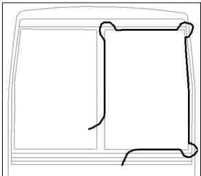
FIGURE 40: WINDSHIELD INSTALLATION USING ROPE
