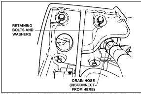
FIGURE 21: ALTERNATOR RETAINING BOLTS AND WASHERS 06350
