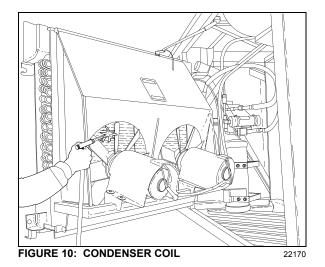
**Caution:** Direct the pressure straight through the coil to prevent bending of fins and do not use extremely high pressure. Do not use hot water, steam or caustic soap.
