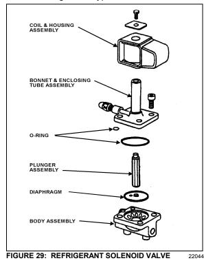
**Caution:** Be careful not to damage the machined faces while the valve is apart.
