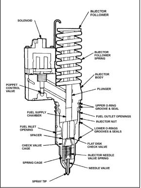
FIGURE 3: UNIT INJECTOR CROSS SECTION
