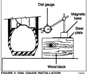
FIGURE 3: DIAL GAUGE INSTALLATION
