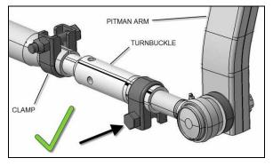
Note horizontal orientation of clamp bolt and bolt insertion direction.
