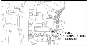
FIGURE 6: FUEL TEMPERATURE SENSOR
