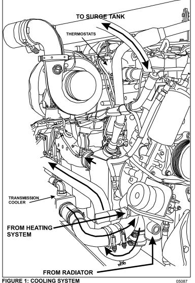
FIGURE 1: COOLING SYSTEM
