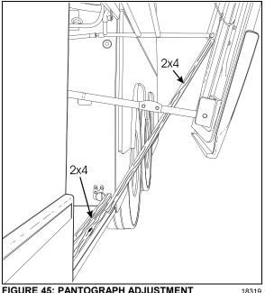
FIGURE 45: PANTOGRAPH ADJUSTMENT
