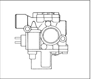
FIGURE 44: ABS MODULATOR VALVE
