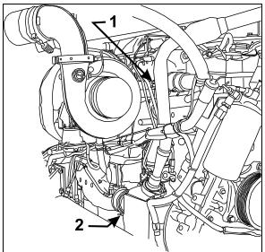
FIGURE 6: ENGINE COOLANT DRAIN COCKS 05088
