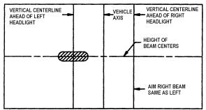
FIGURE 41: HIGH-INTENSITY ZONE (SHADED AREA) OF A PROPERLY AIMED UPPER BEAM ON THE AIMING SCREEN 7.6 M (25FT) IN FRONT OF VEHICLE 06503
