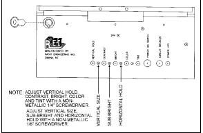
FIGURE 12: MONITOR HOUSING REAR PANEL
