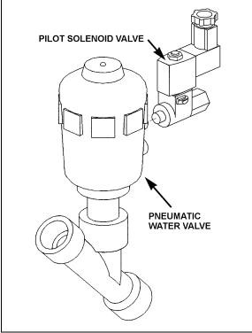
FIGURE 50: CENTRAL HOT WATER PNEUMATIC VALVE ASSEMBLY 22240
