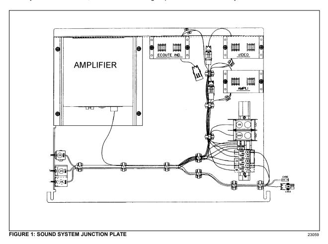
Each service module mounted to the underside of the parcel racks contains a 40-watt speaker. The speakers in the passenger section (twelve in H3-41 or sixteen in H3-45) are wired in stereo and are powered by the amplifier. A microphone outlet mounted in the driver's area is provided as standard equipment.
