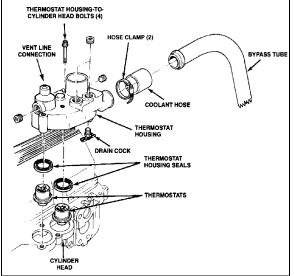
FIGURE 11: THERMOSTAT AND RELATED PARTS 05034
