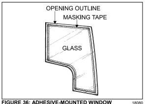
FIGURE 36: ADHESIVE-MOUNTED WINDOW
