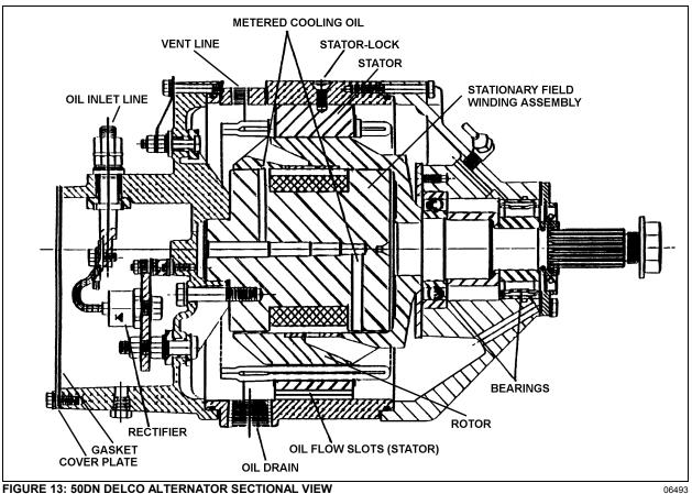
FIGURE 13: 50DN DELCO ALTERNATOR SECTIONAL VIEW
