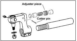
FIGURE 3: TIE-ROD END PLAY ADJUSTMENT
