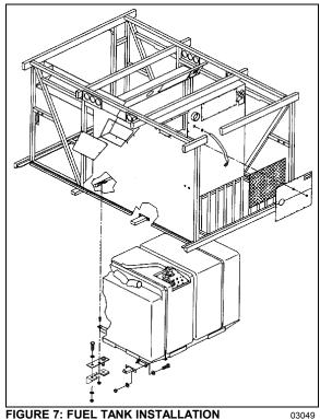
FIGURE 7: FUEL TANK INSTALLATION
