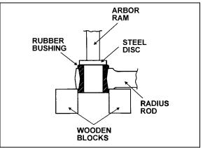
FIGURE 10: RADIUS ROD BUSHING REMOVAL 16011
