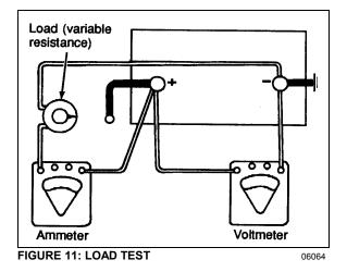
3. With an ammeter reading specified load, read voltage. The voltage should be at least 9.6 volts. Disconnect the load. If the voltmeter indicates 9.6 volts or more, the battery is good. If the voltmeter reading is less than 9.6 volts, replace the battery. This voltage is to be used for battery ambient temperatures of 70°F (21°C) and above. For temperatures below 70°F (21°C), refer to the following "Voltage and Temperature Chart".
