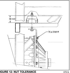
FIGURE 12: NUT TOLERANCE
