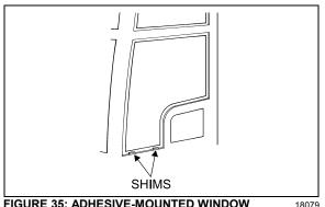
FIGURE 35: ADHESIVE-MOUNTED WINDOW
