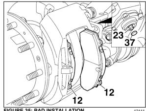
FIGURE 35: PAD INSTALLATION
