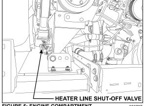
FIGURE 5: ENGINE COMPARTMENT 05078T
