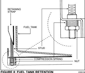
FIGURE 8: FUEL TANK RETENTION
