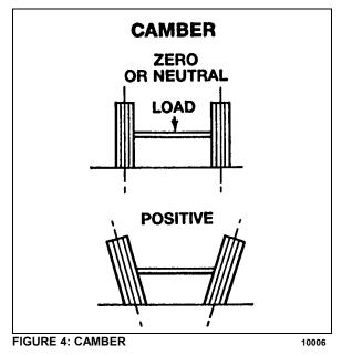
The camber angle is not adjustable. Camber variations may be caused by wear at the wheel bearings, steering knuckle pins or by a bent knuckle or sagging axle center. Steering effort is affected by improper camber, and uneven tire wear will result. Excessive positive camber causes an irregular wear of tire at the outer shoulder and excessive negative camber causes wear at the inner shoulder.
