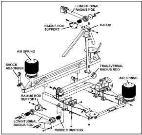
FIGURE 4: DETAILS OF REAR SUSPENSION 16106
