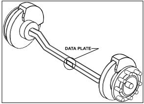
FIGURE 5 : TYPICAL SERIAL AND MODEL NUMBERS10024
