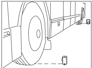
FIGURE 39: INSTALLING CALIBRATION FIXTURES 06497
