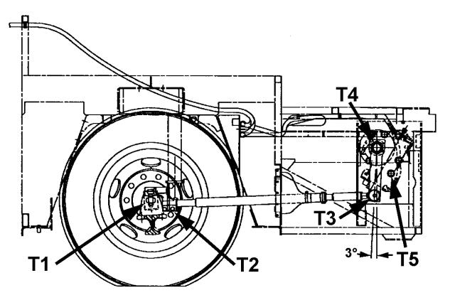
FIGURE 10: DRAG LINK COMPONENTS
