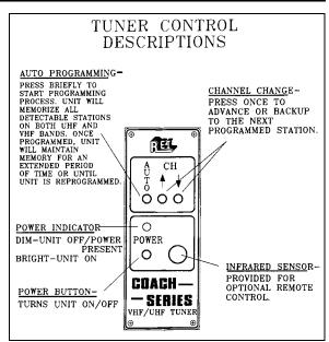
FIGURE 10: TUNER CONTROLS DESCRIPTION
