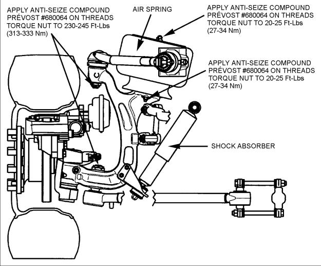
FIGURE 23: AIR SPRING AND SHOCK ABSORBER
