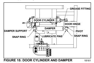
**Caution:** It is important to make sure that damper does not reach end of stroke when door is completely closed or opened. The door cylinder must stop the door on opening. Screw or unscrew rod end to adjust if necessary.
