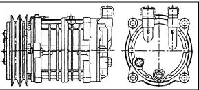
FIGURE 33: SELTEC TM-16HD COMPRESSOR
