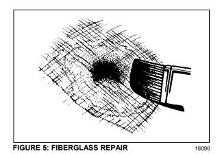
Apply another mat, followed by a cloth patch, and another mat. All layers must be thoroughly impregnated with polyester resin, brushed well and free of air. Apply more layers of mat and cloth as required until the desired strength and thickness is obtained, minimum two 1-1/2 oz (43 g) mats and one 9 oz (255 g) cloth (Fig. 6).
