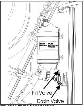
FIGURE 31: REAR VALVE LOCATION
