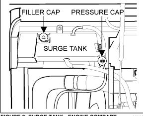
FIGURE 2: SURGE TANK - ENGINE COMPART. 05086
