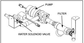
FIGURE 52: VIP WATER RECIRCULATION PUMP INSTALLATION
