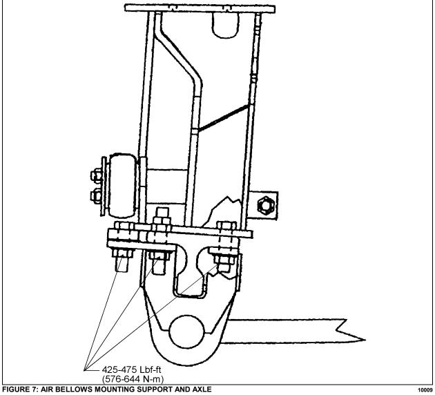
For more torque specifications, see 'Dana Spicer Maintenance Manual NDS Axles and Maintenance Manual Model NDS' annexed at the end of this section.
