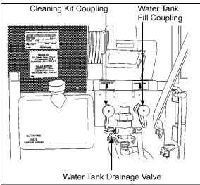
FIGURE 24: FRESH WATER TANK SERVICE VALVES
