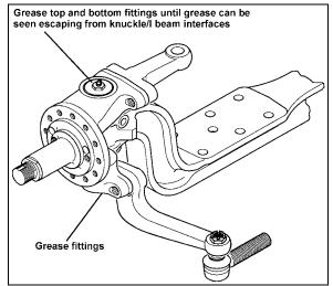
FIGURE 2: FRONT AXLE GREASING POINTS
