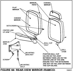
FIGURE 66: REAR-VIEW MIRROR (RAMCO)
