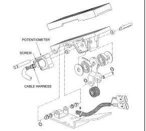
FIGURE 8: ELECTRONIC FOOT PEDAL ASSEMBLY 03035
