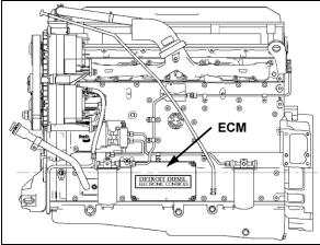
FIGURE 2: ELECTRONIC CONTROL MODULE (ECM) 01064
