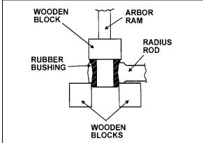
FIGURE 11: RADIUS ROD BUSHING INSTALLATION 16012
