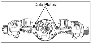
FIGURE 4: TYPICAL SERIAL & MODEL NUMBERS 11019
