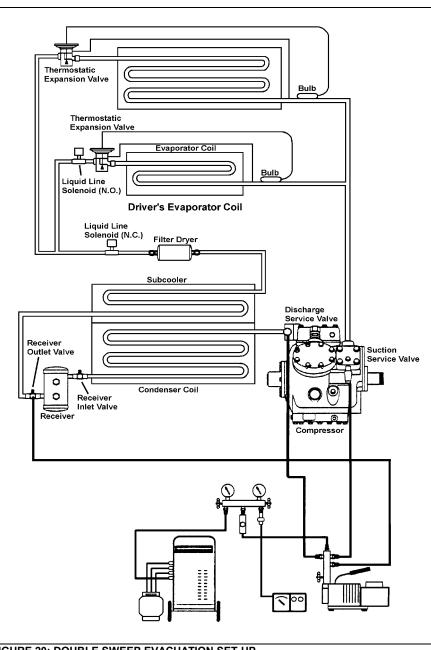
FIGURE 20: DOUBLE SWEEP EVACUATION SET-UP
