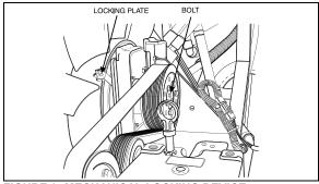
FIGURE 9: MECHANICAL LOCKING DEVICE 05061
