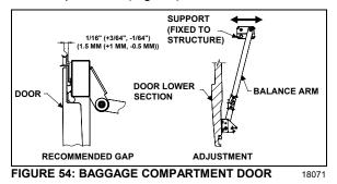
Once the adjustment procedure is achieved, ensure that all bolts are securely tightened.
