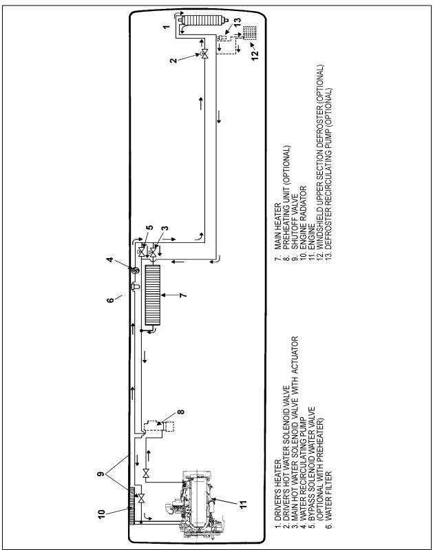
FIGURE 47: CENTRAL HEATING SYSTEM COMPONENTS
