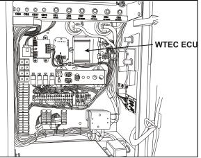
FIGURE 14: WTEC / ELECTRONIC CONTROL UNIT 07075
