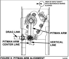
FIGURE 8: PITMAN ARM ALIGNMENT
