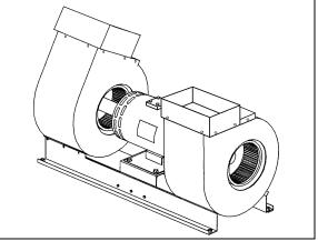
FIGURE 17: EVAPORATOR MOTOR ASSEMBLY 22228
