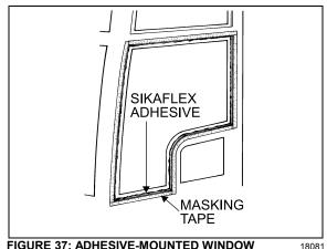
FIGURE 37: ADHESIVE-MOUNTED WINDOW
