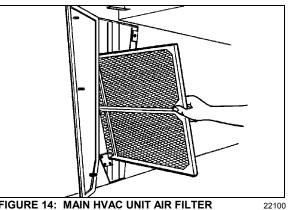
FIGURE 14: MAIN HVAC UNIT AIR FILTER
