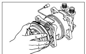
FIGURE 36: ROTATING MAGNETIC CLUTCH
