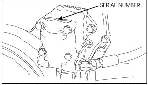
FIGURE 7 : POWER STEERING PUMP SERIAL NUMBER
