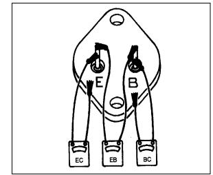
FIGURE 28: CHECKING TRANSISTORS TR1
