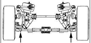
FIGURE 69: JACKING POINTS ON IND. SUSPENSION
