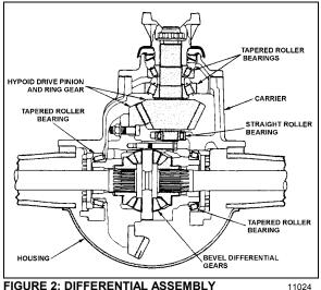
FIGURE 2: DIFFERENTIAL ASSEMBLY
