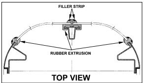
FIGURE 39: WINDSHIELD INSTALLATION TOP VIEW18098
