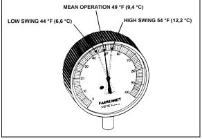
FIGURE 32: HIGH & LOW SWING TEMPERATURE AT REMOTE BULB 22047
