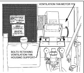
FIGURE 22: VENTILATION FAN INSTALLATION
