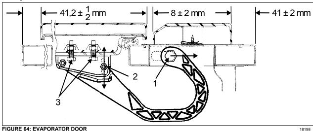
FIGURE 64: EVAPORATOR DOOR
