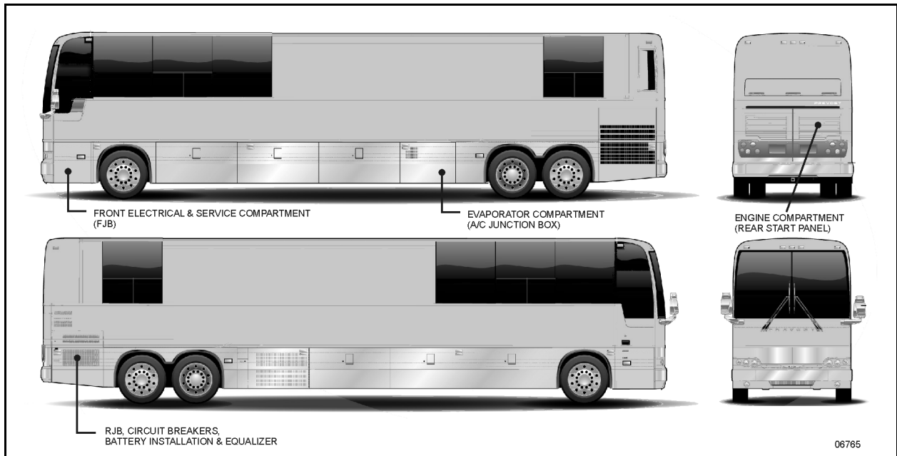
FIGURE 14: ELECTRICAL COMPARTMENTS (X3-45 VIP)
