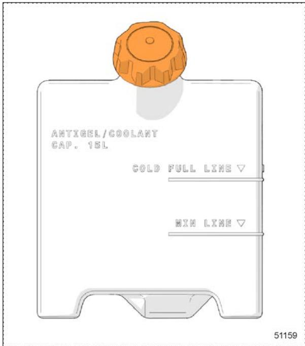
Fill the recovery tank with the same 50/50 water-antifreeze mixture already in the cooling system. Do not mix two different types of coolant. Refer to the Maintenance Manual for proper coolant type specifications or see the label affixed near the coolant surge tank on the vehicle.
