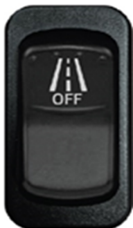
FIGURE 16: LDW ENABLE/DISABLE SWITCH
