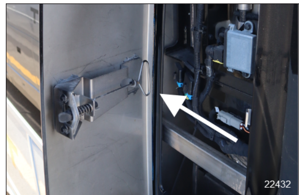
FIGURE 37: SCR ACCESS DOOR HANDLE
