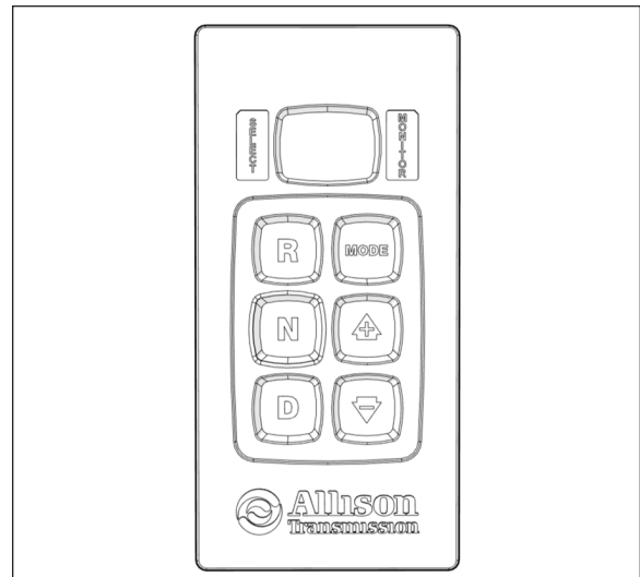
FIGURE 5: TRANSMISSION CONTROL PAD
