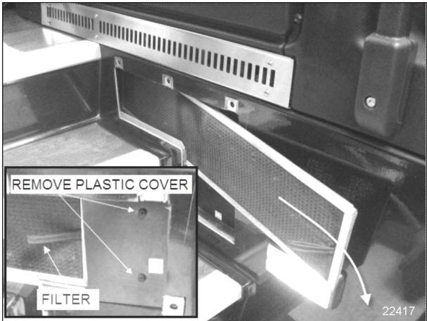
FIGURE 21: REMOVING DRIVER'S SECTION AIR FILTER
