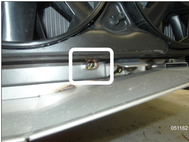
FIGURE 11: FAN SHROUD TOP & BOTTOM HOLD-DOWN SCREWS
