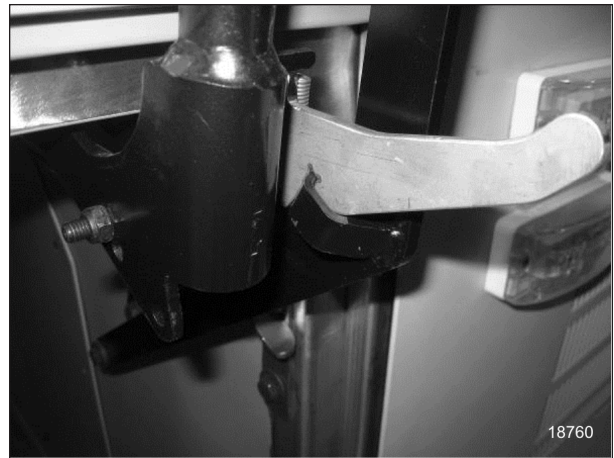
FIGURE 22: BAGGAGE DOOR LOCK AND LEVER
