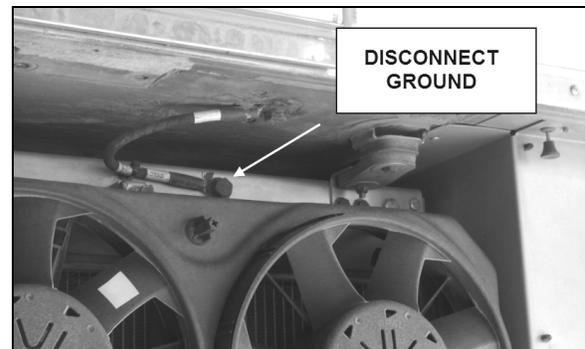
FIGURE 32: COOLING ASSEMBLY GROUND
