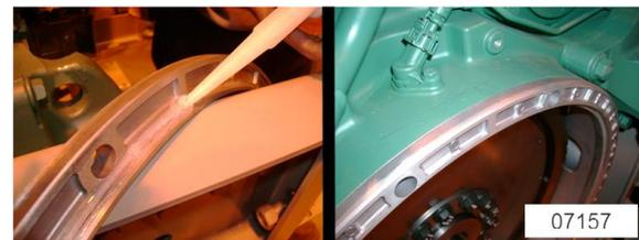
FIGURE 11: SPACER INSTALLATION
