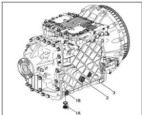
FIGURE 17: I-SHIFT TRANSMISSION OIL CHANGE
