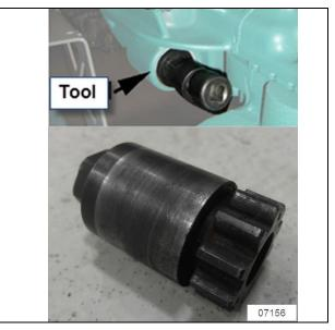
FIGURE 10: VOLVO ENGINE TURNING TOOL #88800014
