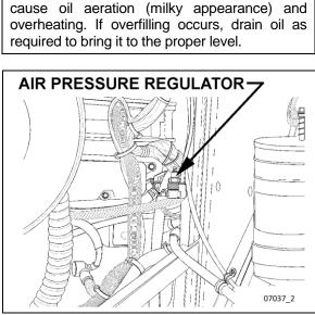
FIGURE 14: AIR PRESSURE REGULATOR (TYPICAL)
