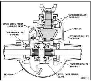
FIGURE 2: DIFFERENTIAL ASSEMBLY
