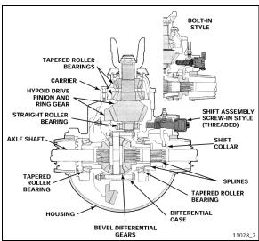
FIGURE 3: DRIVER-CONTROLLED DIFFERENTIAL LOCK
