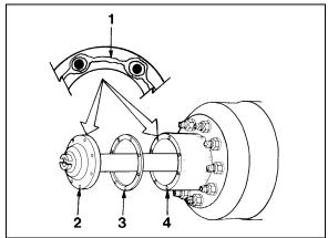
FIGURE 8: AXLE SHAFT INSTALLATION
