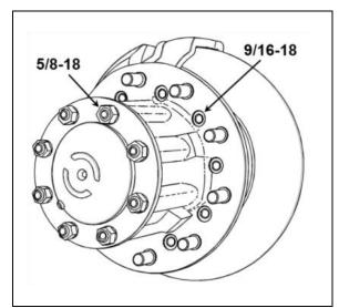
FIGURE 9: FASTENER SIZE IDENTIFICATION
