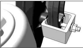
FIGURE 15: INSTALLING EXTRACTOR TOOL
