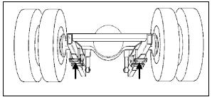
FIGURE 6: JACKING POINTS ON DRIVE AXLE
