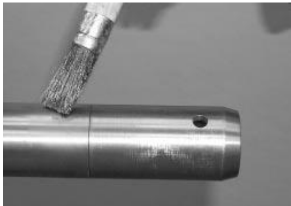
FIGURE 10: APPLY GLEITMO 805 GREASE
