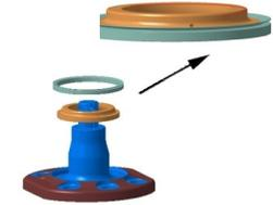
6. Install backup ring and dust boot on bell crank or idler arm spindle.
