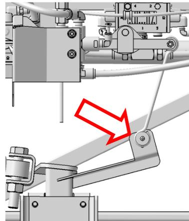
5. Loosen the lower mounting bolt shown.
