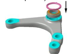
5. Apply good quality lithium grease (#680752) on backup ring and dust boot.
