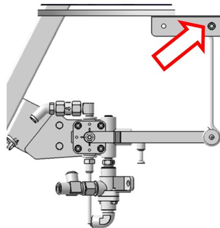
5. Loosen the lower mounting bolt shown.
