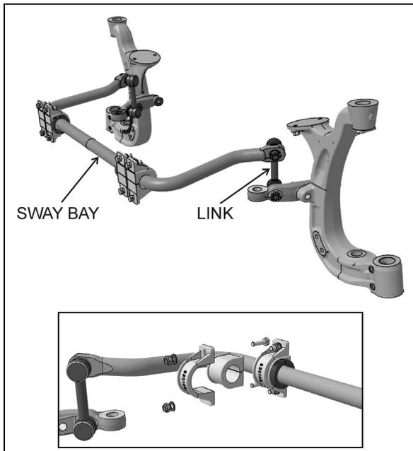
**FIGURE 34: SWAY BAR (INDEPENDENT FRONT SUSPENSION)**
