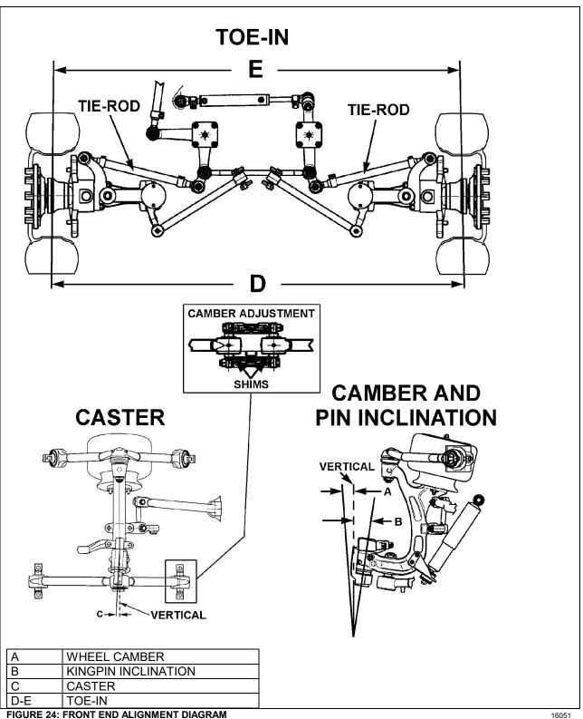
FIGURE 24: FRONT END ALIGNMENT DIAGRAM
