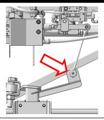
5. Loosen the lower mounting bolt shown.
