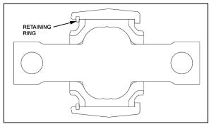
FIGURE 28: UPPER A-ARM BALL PIN BUSHING
