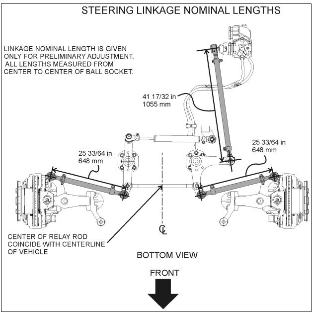
FIGURE 19: STEERING LINKAGE NOMINAL LENGTHS
