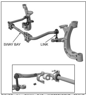
FIGURE 34: SWAY BAR (INDEPENDENT FRONT SUSPENSION) FRONT
