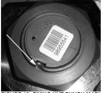
FIGURE 13: FIXING NUT PUNCH MARK
