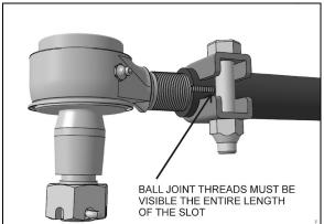
FIGURE 21: ADEQUATE CLAMPING CONDITION
