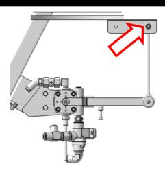
5. Loosen the lower mounting bolt shown.
