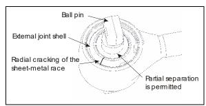
FIGURE 7: BALL PIN BUSHING
