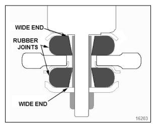
FIGURE 33: LOWER SHOCK MOUNTING BUSHINGS
