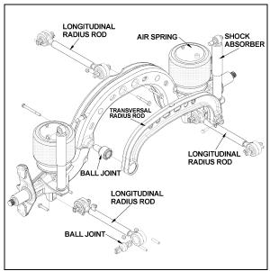
**FIGURE 36: TAG AXLE SUSPENSION**
