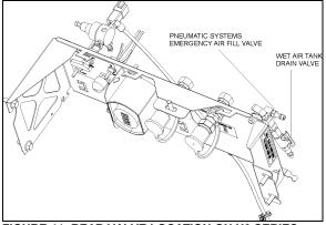
FIGURE 44: REAR VALVE LOCATION ON H3 SERIES 12162
