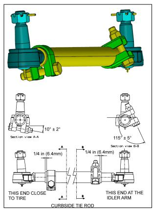
FIGURE 17: CURBSIDE TIE ROD - CLAMPS POSITION 16199
