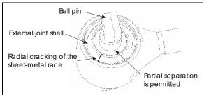
**FIGURE 26: BALL PIN BUSHING**
