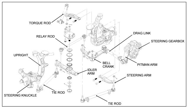
FIGURE 10: IFS STEERING LINKAGE OVERVIEW
