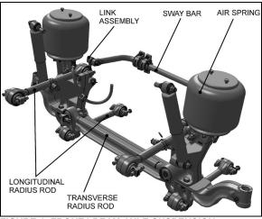
FIGURE 1: FRONT I-BEAM AXLE SUSPENSION
