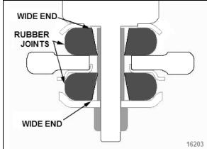
FIGURE 40: LOWER SHOCK MOUNTING BUSHINGS
