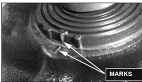
FIGURE 11: STEERING GEARBOX INPUT SHAFT MARKS
