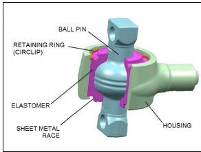
FIGURE 6: BALL PIN JOINT CONSTRUCTION
